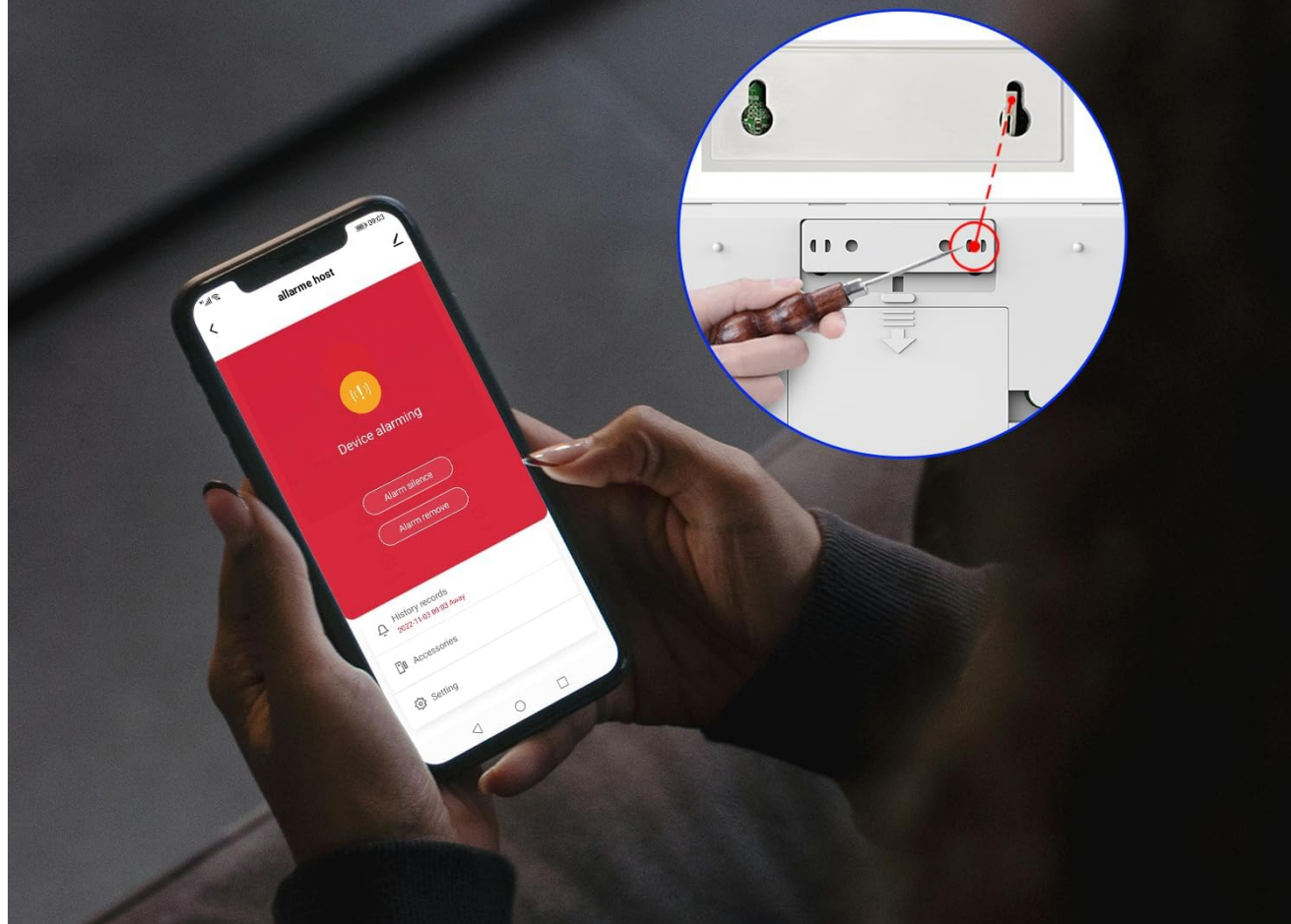
Figure 3: The anti-demolition alarm feature on the back of the main unit. If removed, an alarm will sound and a notification will be sent.
