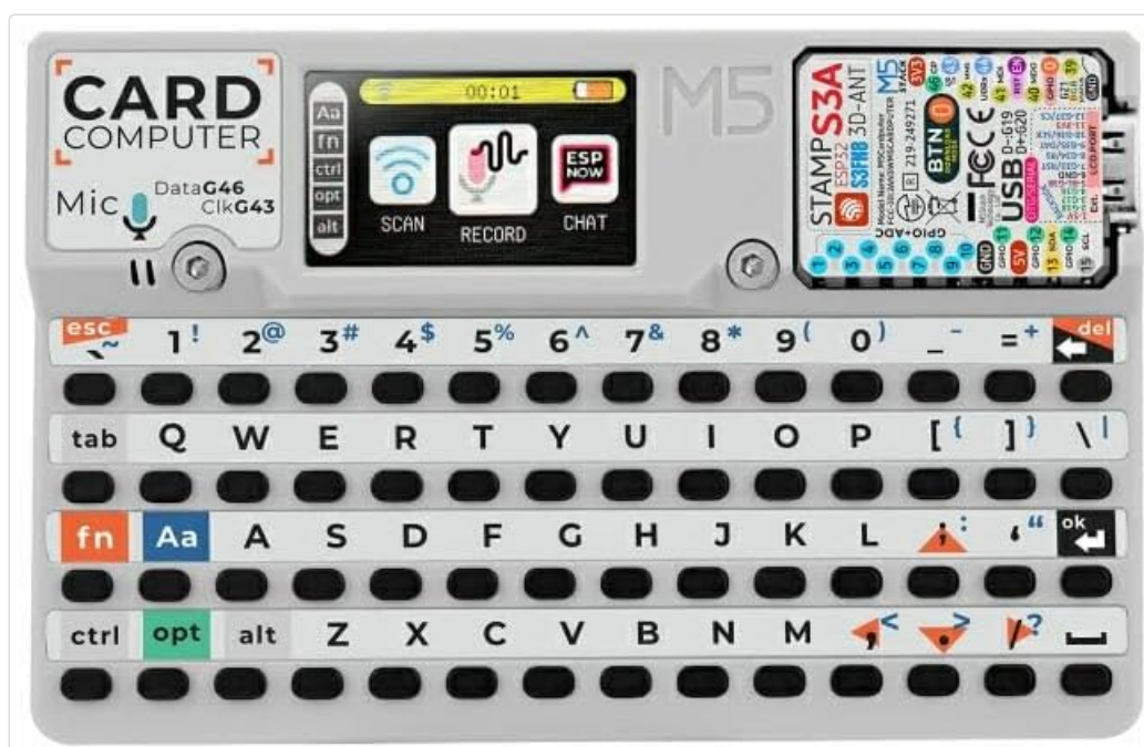
Figure 3.2: Detailed overview of the Cardputer v1.1 components, including the 1.14-inch IPS-LCD, 56-key keyboard, StampS3A microcontroller, speaker, microphone, IR emitter, Micro SD slot, and battery specifications.
