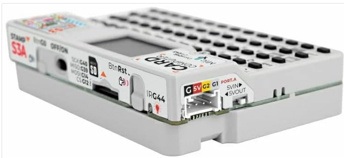
Figure 3.4: Side view illustrating the Grove interface (HY2.0-4P), Micro SD card slot, and reset button.
