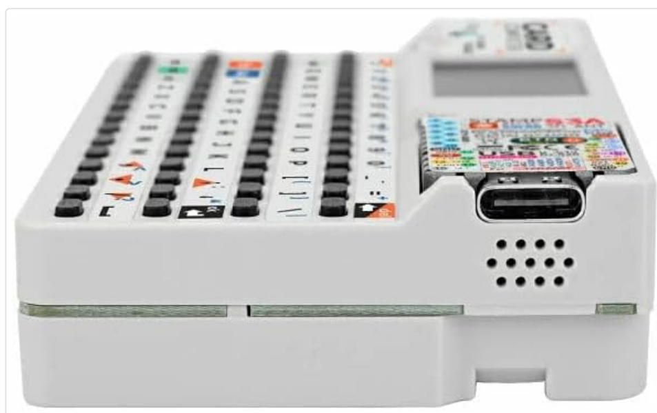
Figure 3.5: Opposite side view of the Cardputer v1.1, highlighting the USB-C port for power and data transfer.
