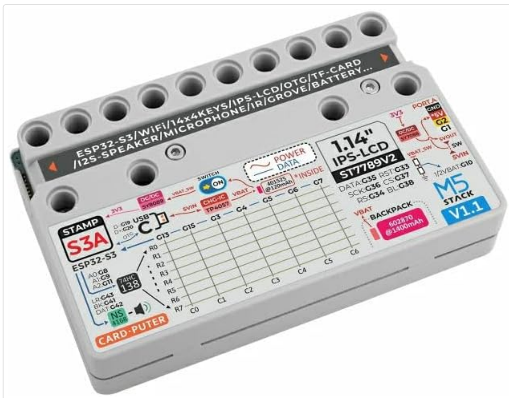
Figure 3.7: Rear view of the Cardputer v1.1, showing the base with integrated 1400mAh battery and LEGO stud compatibility.
