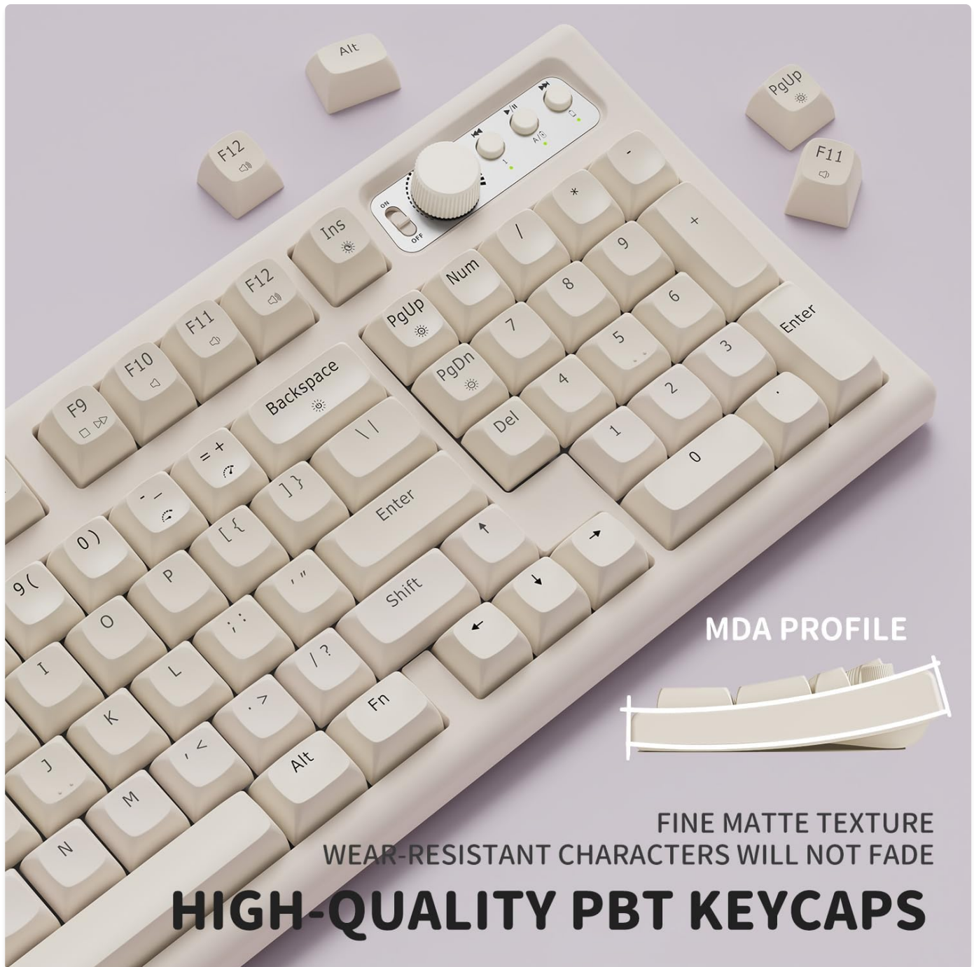
Image: Close-up of the keyboard's high-quality PBT keycaps with MDA profile, highlighting their fine matte texture and wear-resistant characters.
