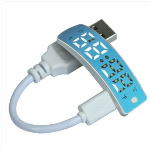
Image: The e-vibra W15 watch module plugged into a USB port for charging.
