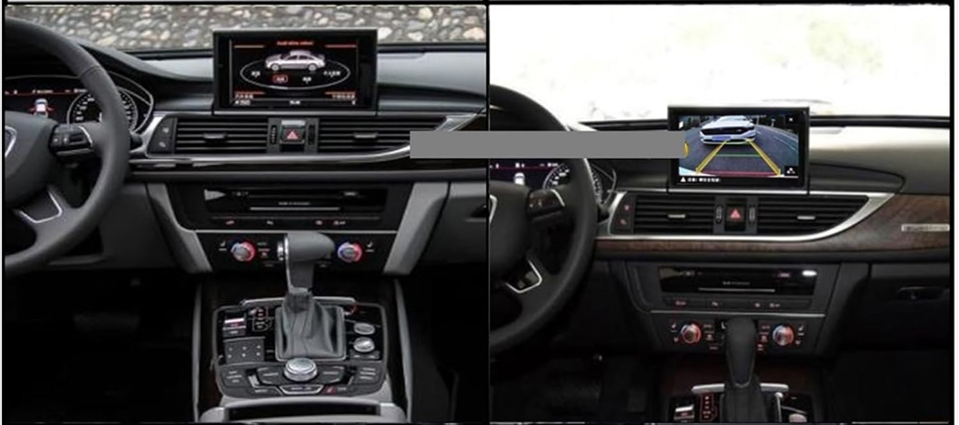
Figure 3.1: Visual comparison showing the car's screen before and after the reversing camera system is installed, displaying the new reversing image.
