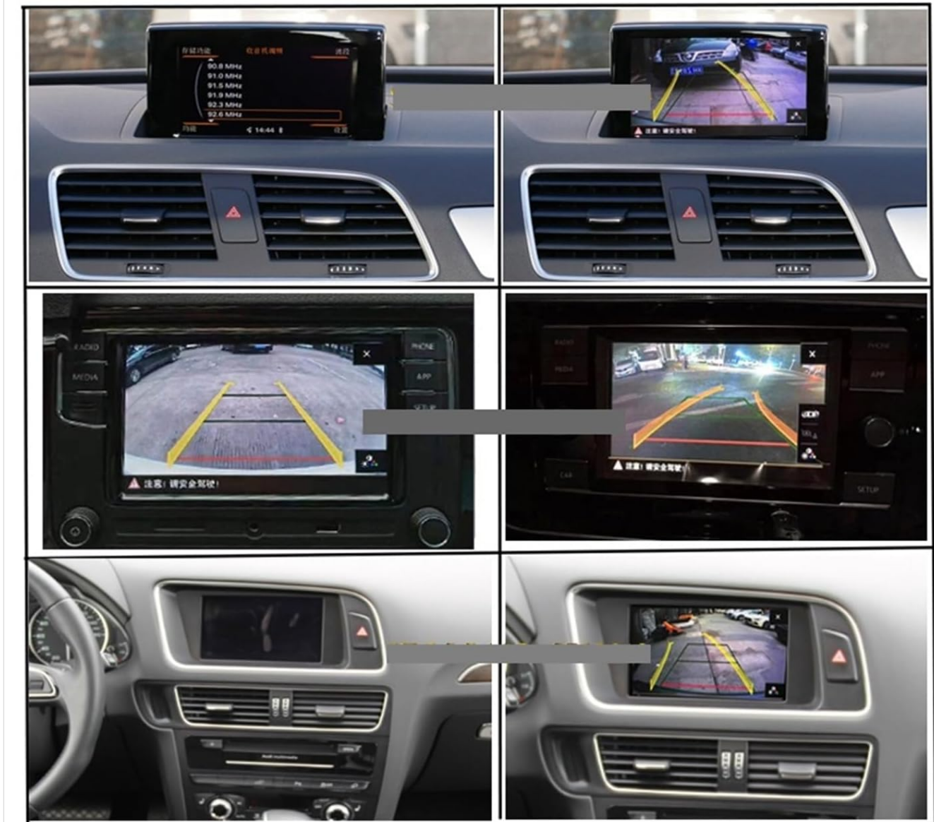
Figure 4.1: Examples of the camera's output displayed on different car screens, demonstrating the clear image quality and dynamic trajectory lines that assist with parking.
