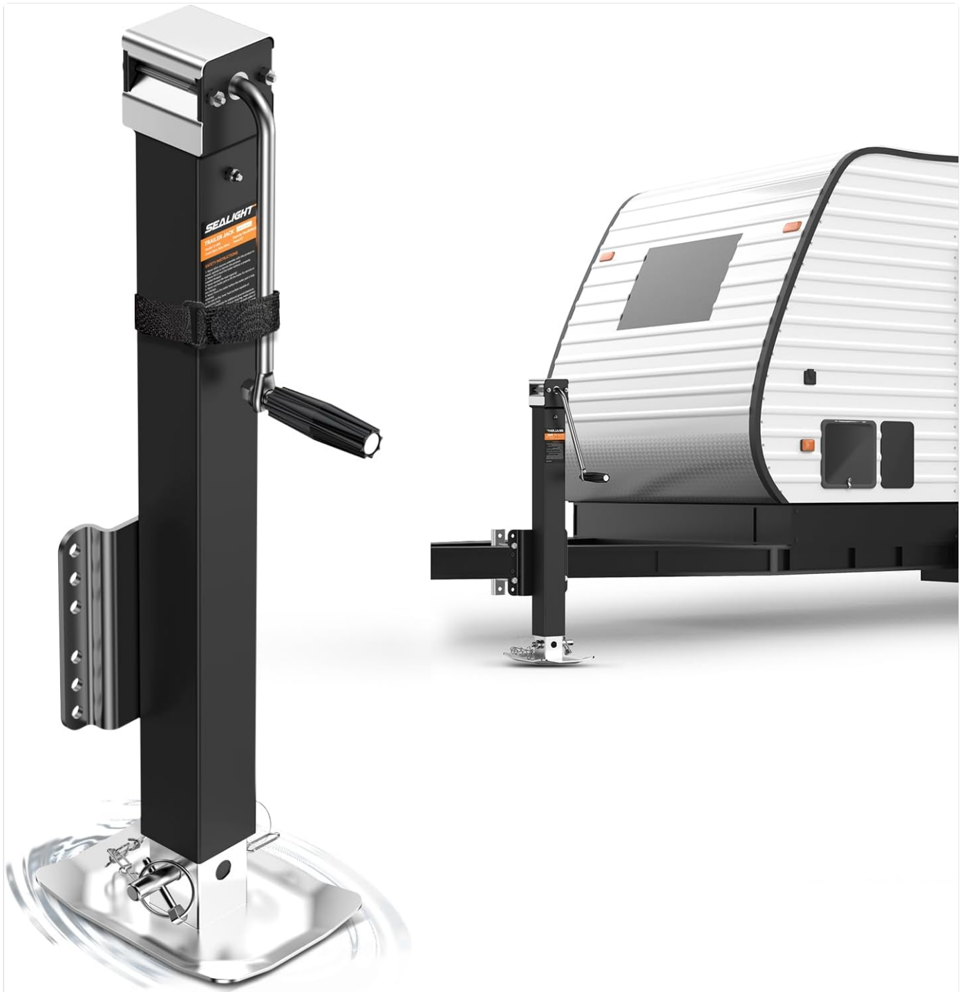
Image 3.1: The SEALIGHT 8000LBS Heavy-Duty Trailer Jack positioned next to a trailer, illustrating its robust construction and intended application. The jack features a hand-crank mechanism and a wide base for stability.
