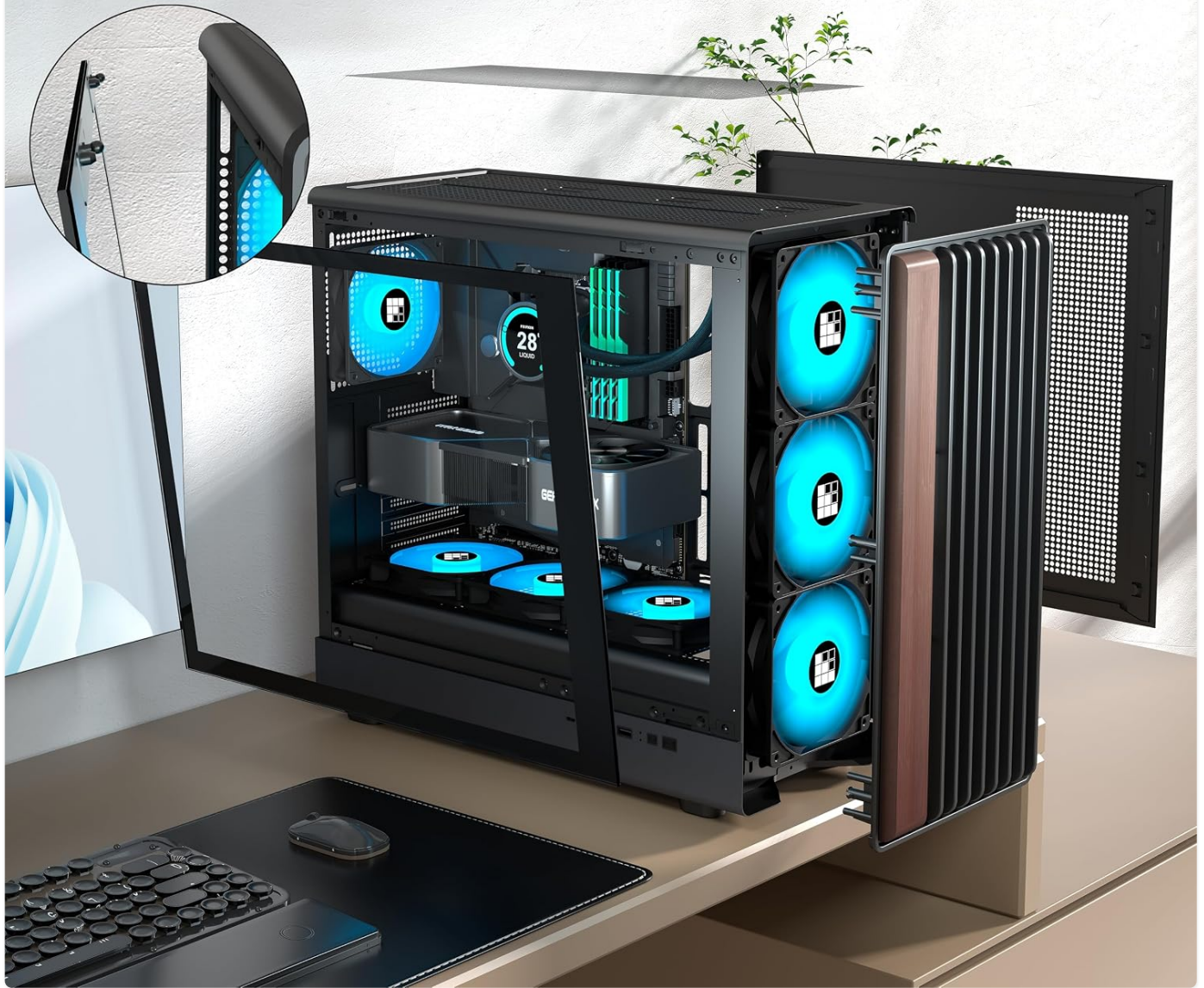
Image: Demonstrating the tool-less removal of the tempered glass side panel.
