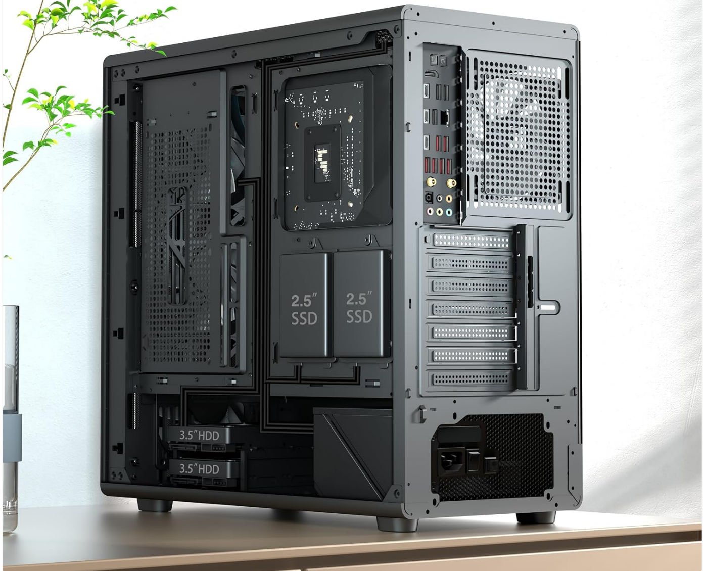
Image: Rear view of the case showing cable management routes and storage drive mounting points.
