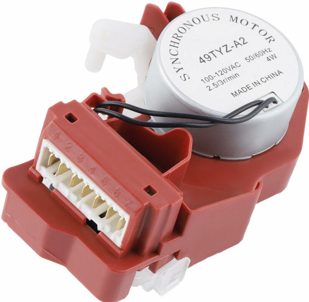
**Figure 1:** Whirlpool Washer Shift Actuator Replacement Part. This image displays the replacement shift actuator. It features a red plastic housing with a silver synchronous motor attached. The motor label indicates specifications such as 100-120VAC, 50/60Hz, 4W, and 2.5/3r/min, with model number 49TYZ-A2 and 'MADE IN CHINA'.
