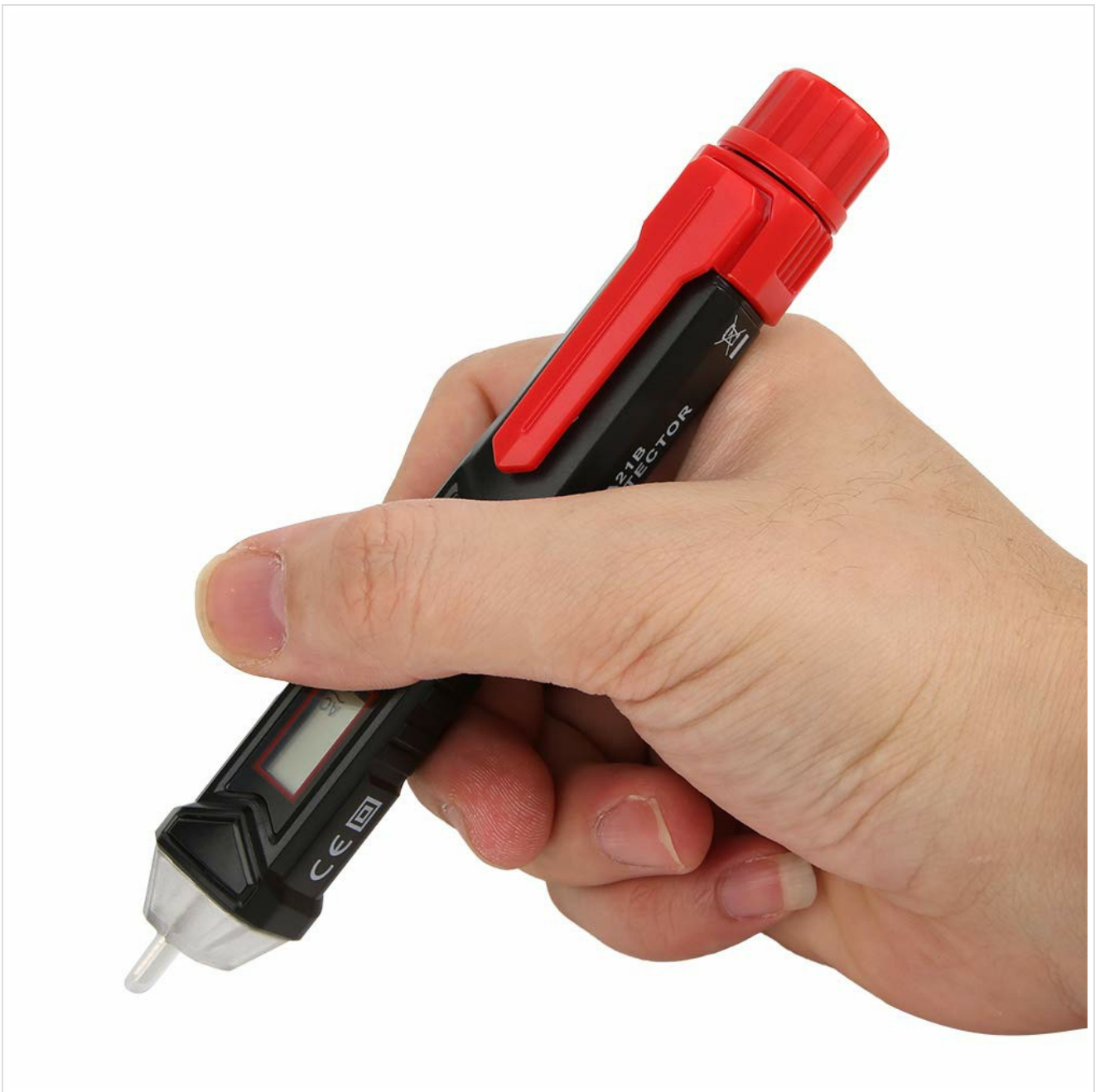
Figure 5.1: Demonstrating the SASKATE TA11B Voltage Tester being held for non-contact testing.
