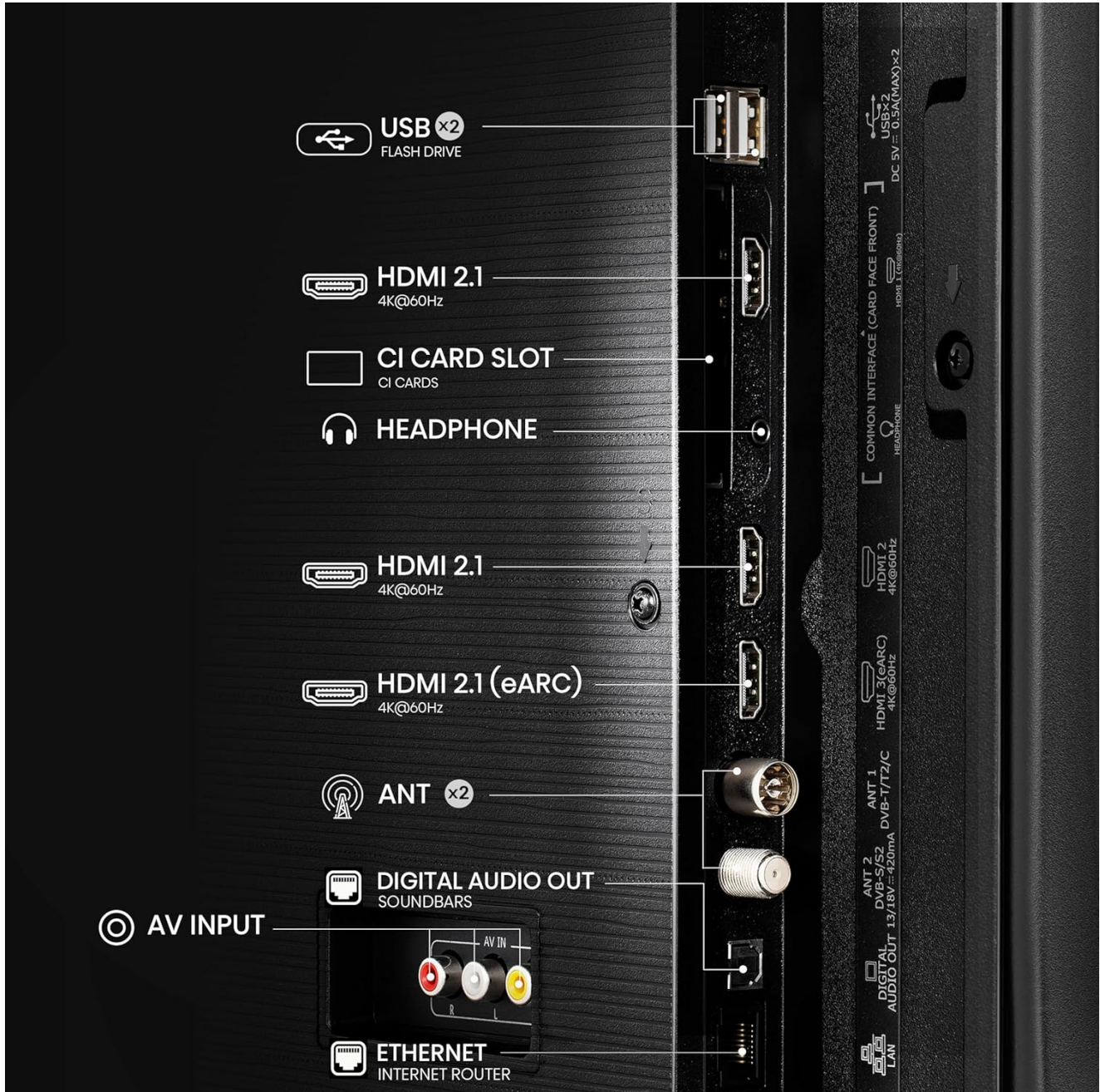
Image: Detailed view of the Hisense 55E78Q TV's rear panel, highlighting various input and output ports including USB (x2), HDMI 2.1 (x3, one with eARC), CI Card Slot, Headphone, ANT (x2), Digital Audio Out, AV Input, and Ethernet.
