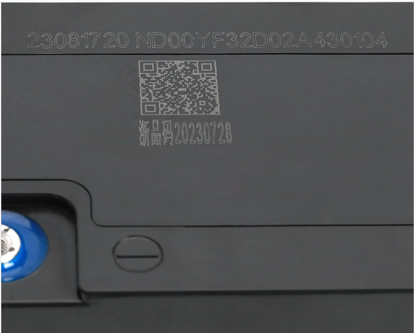
Figure 6.1: QR code and serial number on the battery for product information. Link: http://www.pzcode.cn/pwb/3146762023081720ND00YF32D02A430104
