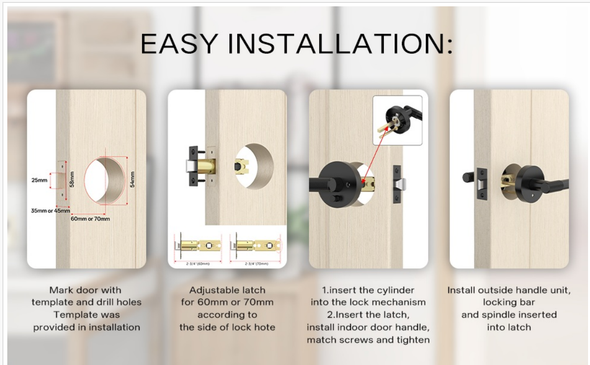
Image: A four-step visual guide demonstrating the installation process: marking and drilling holes, adjusting the latch, inserting the cylinder and indoor handle, and installing the outside handle unit with the locking bar and spindle.
