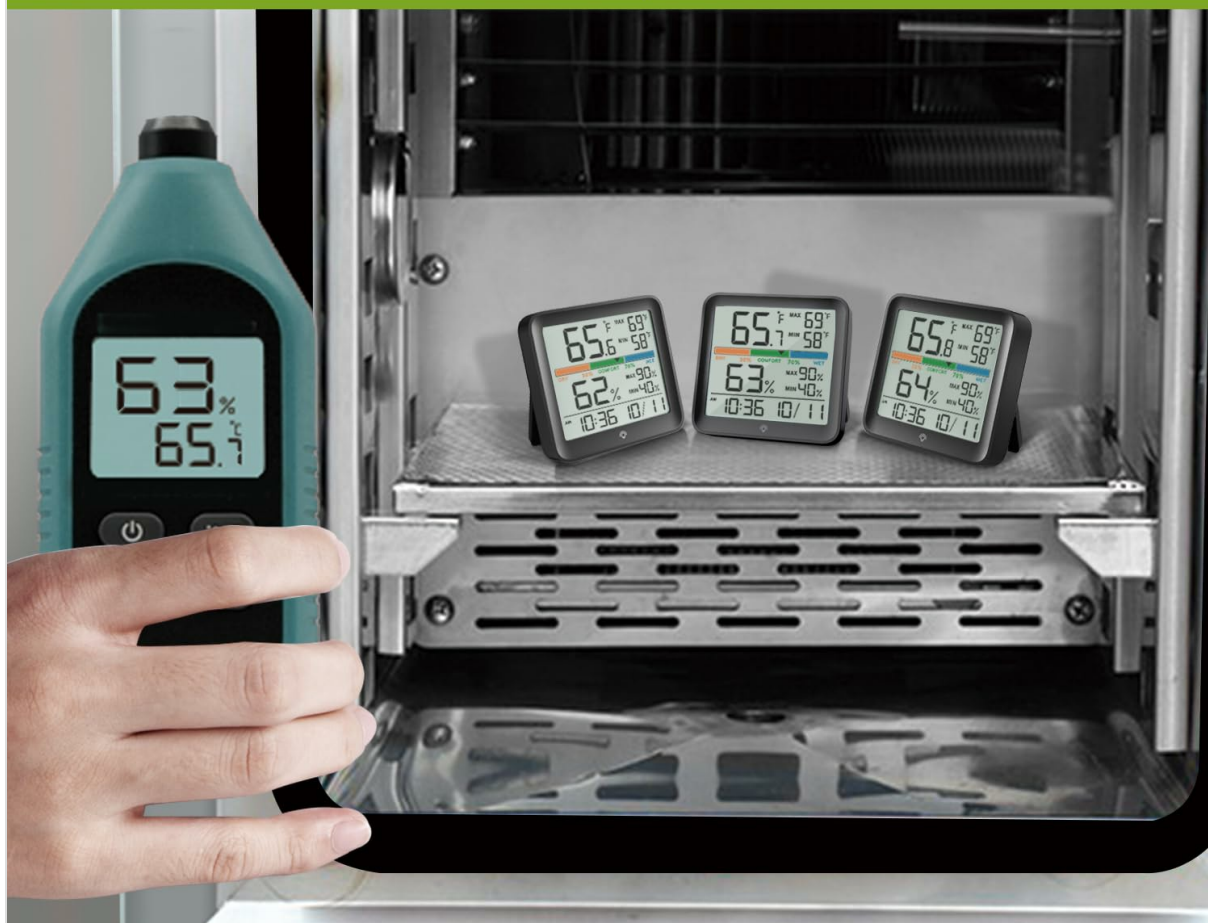
Image: Illustration of the calibration process, showing the device being compared to other measurement tools for accuracy adjustment.
