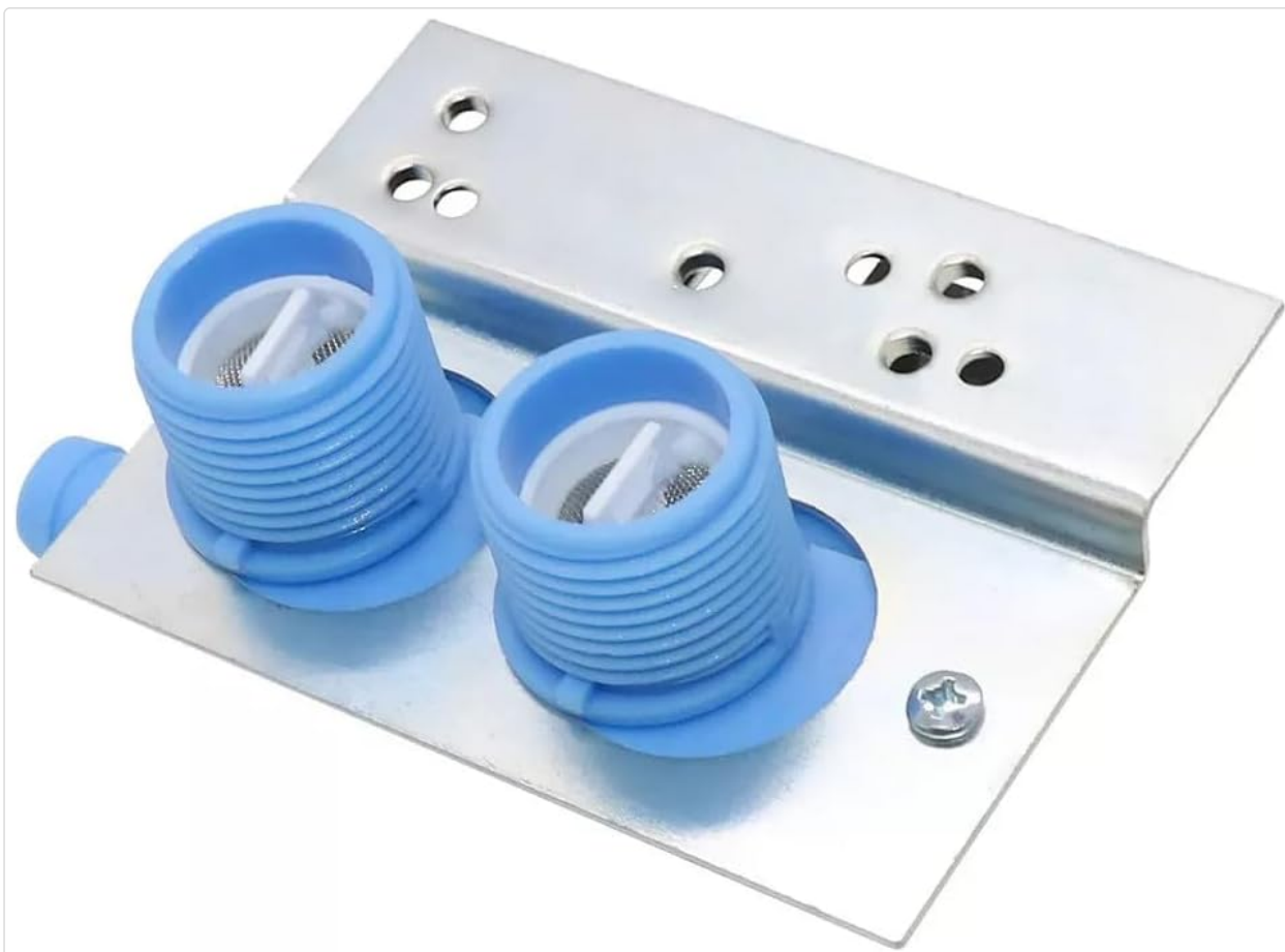
Figure 3: Underside view of the valve, revealing the two threaded water outlet connections. Each connection includes a fine mesh filter to prevent sediment from entering the washing machine.
