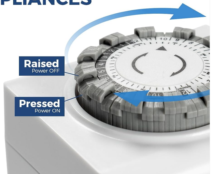
Figure 5: Mechanical Timer Operation
