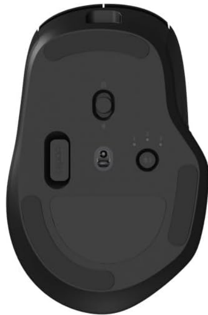
Figure 4: Bottom view of the mouse, showing the optical sensor, power switch, and mode selection button.
