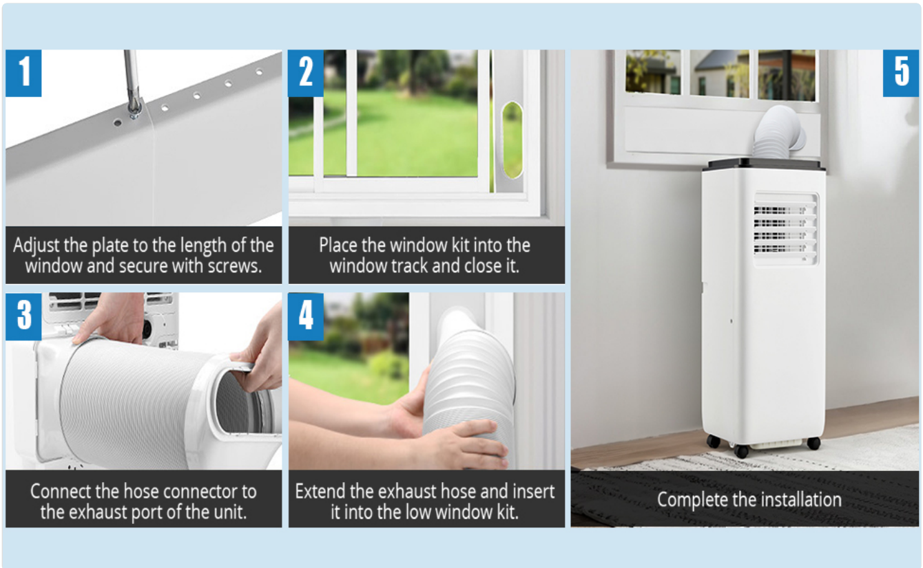
Image: A visual guide illustrating five steps for installing the window kit: adjusting the plate, placing it in the window track, connecting the hose to the unit, extending the hose to the window kit, and showing the complete installation.
