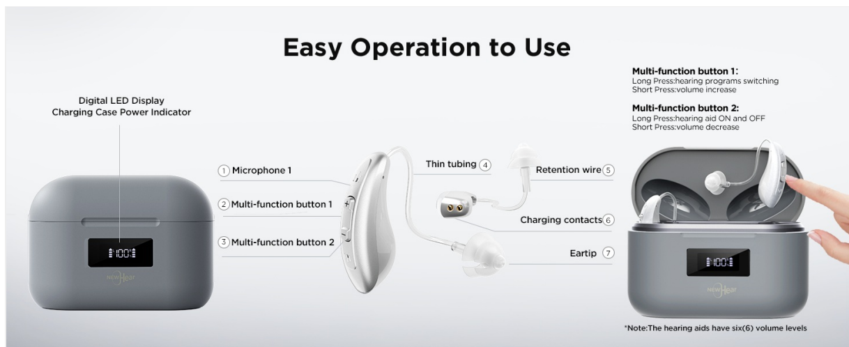
Image: Detailed diagram of the hearing aid components and charging case.
