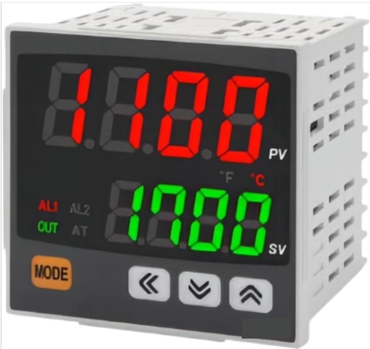
Image Description: This image displays the front panel of the Mechanivis TCN4M-22R Temperature Controller. It features a red digital display for the Process Value (PV) and a green digital display for the Set Value (SV). Below the displays are indicators for AL1 (Alarm 1), AL2 (Alarm 2), OUT (Output), and AT (Auto-tuning). Control buttons include 'MODE' and three arrow keys for navigation and adjustment.
