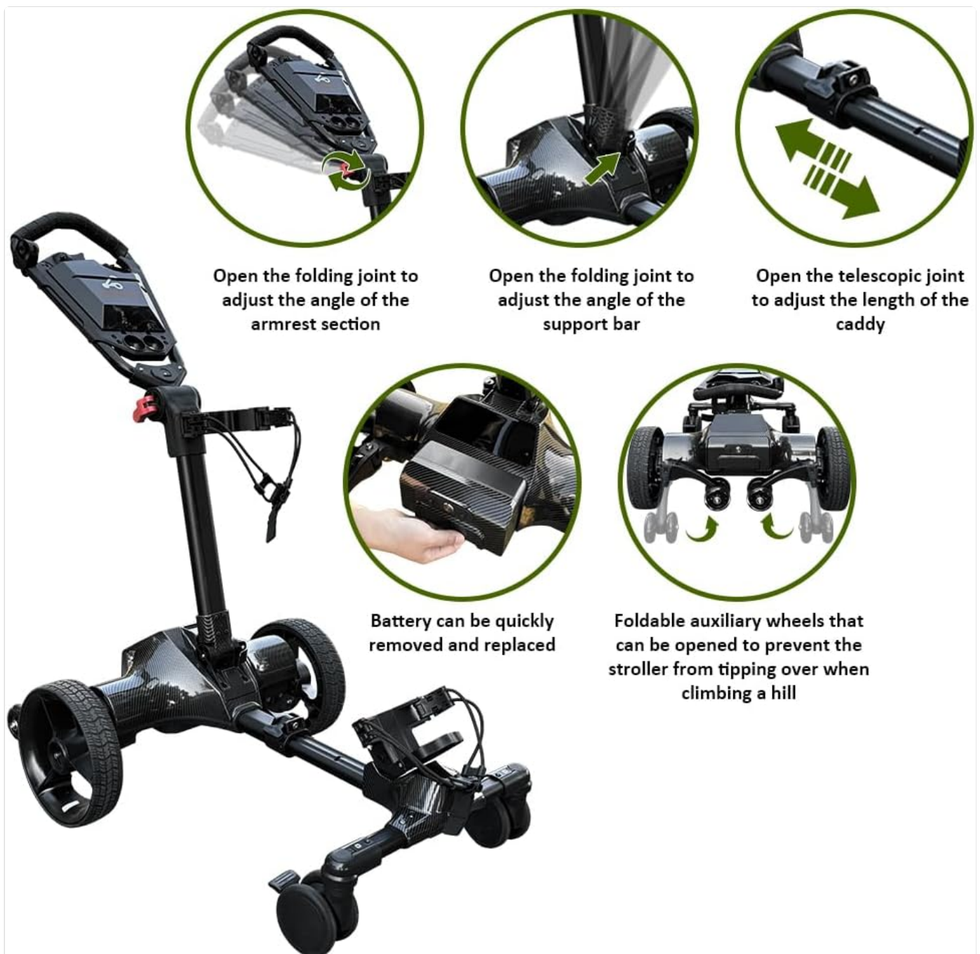
Figure 9: Visual guide to collapsing the G3 Electric Golf Cart.
