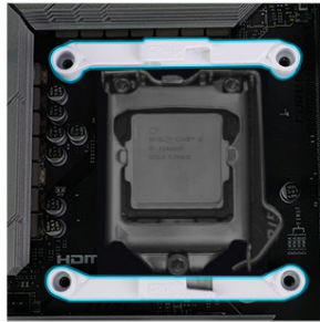
2. Mount the water block bracket, ensuring the notch is aligned to the right.
