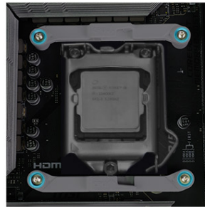
3. Use the included screwdriver to secure the bracket screws—again, ensure the notch is on the right.
