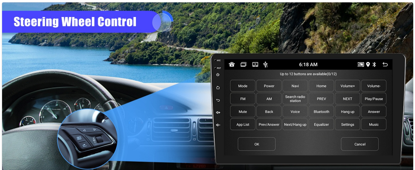
Figure 11: Steering Wheel Control mapping interface.
