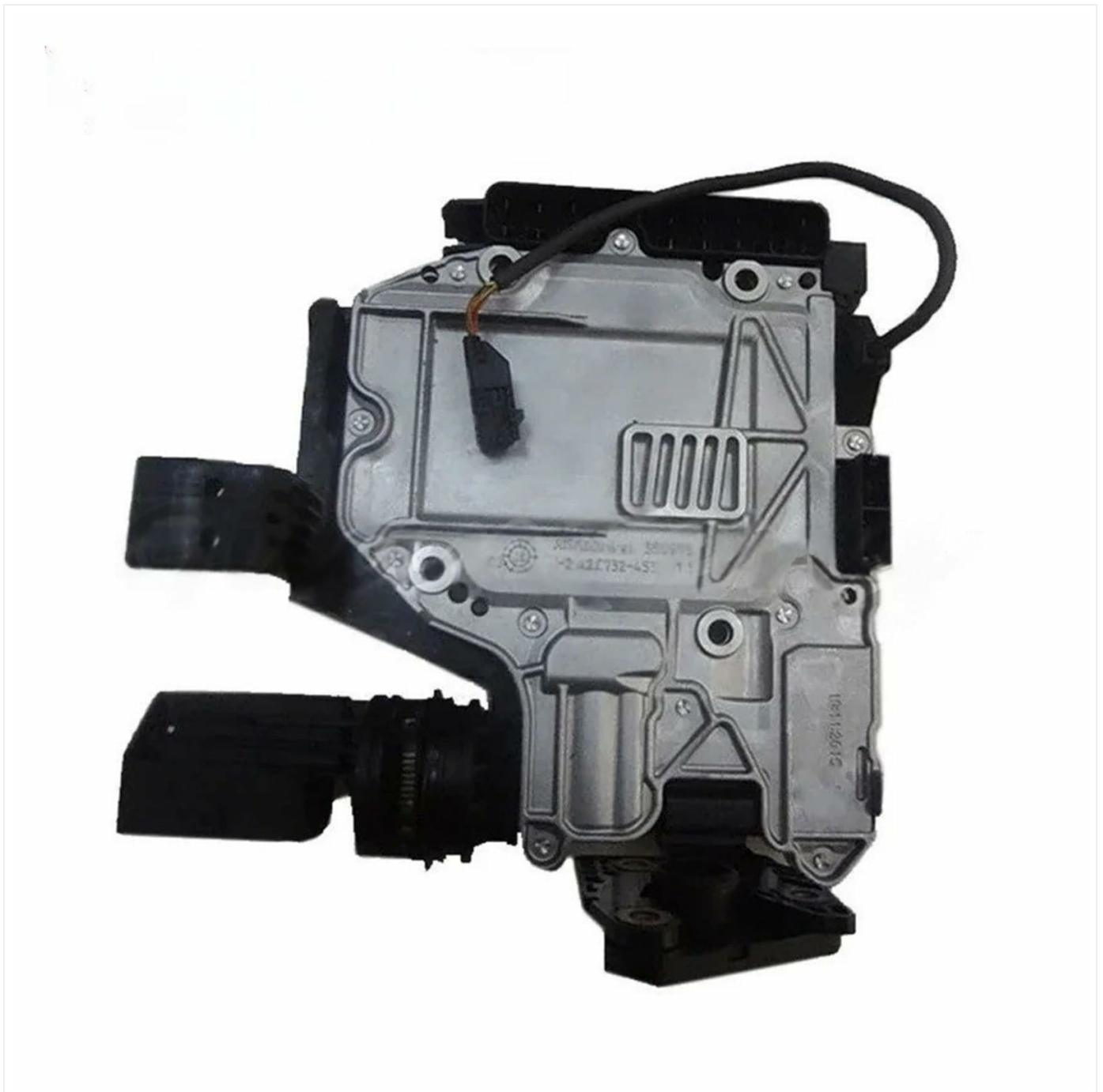
Figure 1: Front view of the 0CK DL382 Transmission Control Unit Module, showing its robust casing and electrical connectors.
