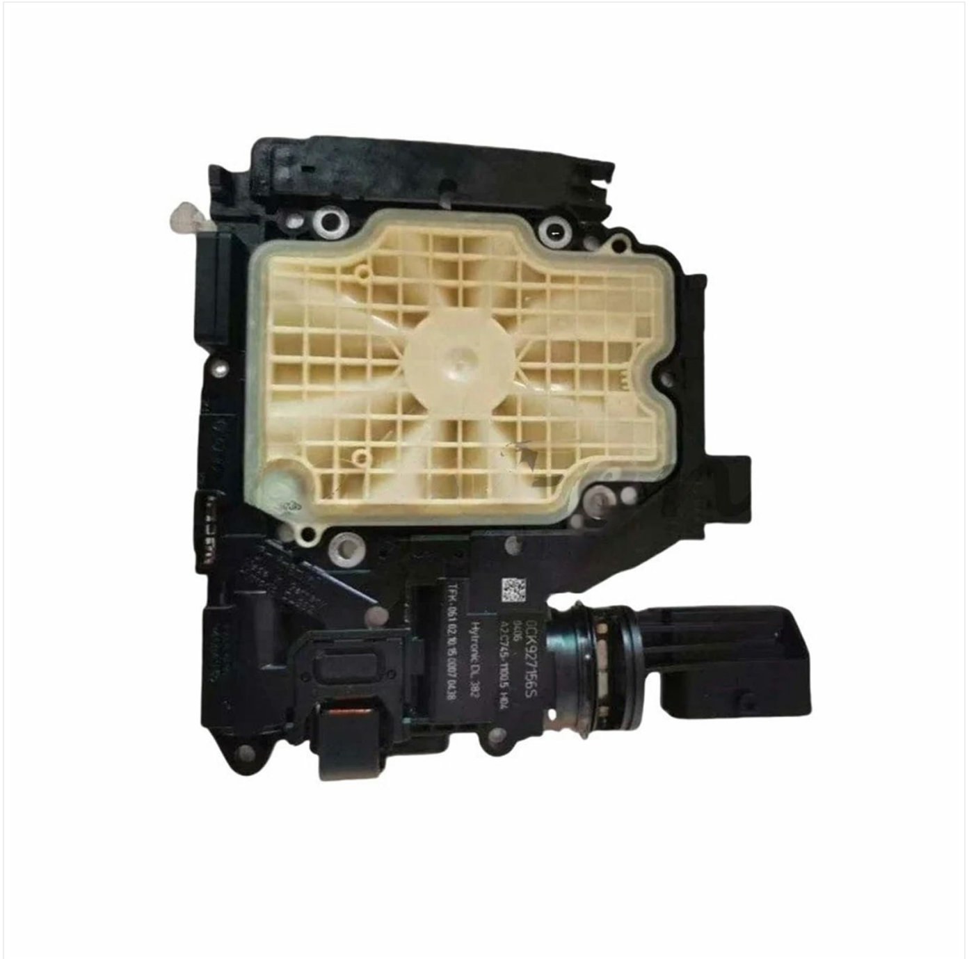
Figure 3: Internal view of the 0CK DL382 TCU, showing the valve body and mechatronic components under a protective cover, highlighting the intricate design.
