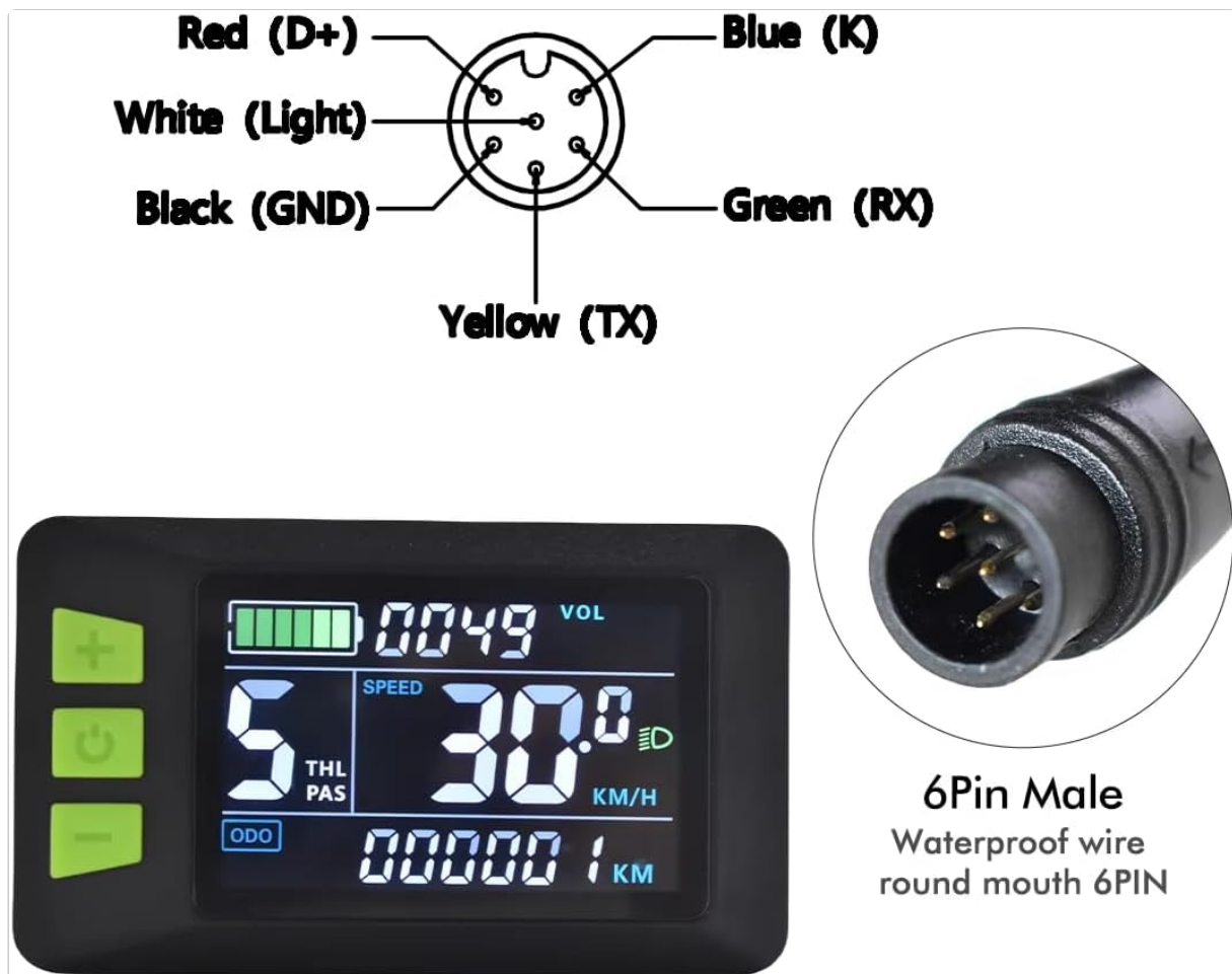
Figure 3: 6PIN Connector Wiring Diagram
