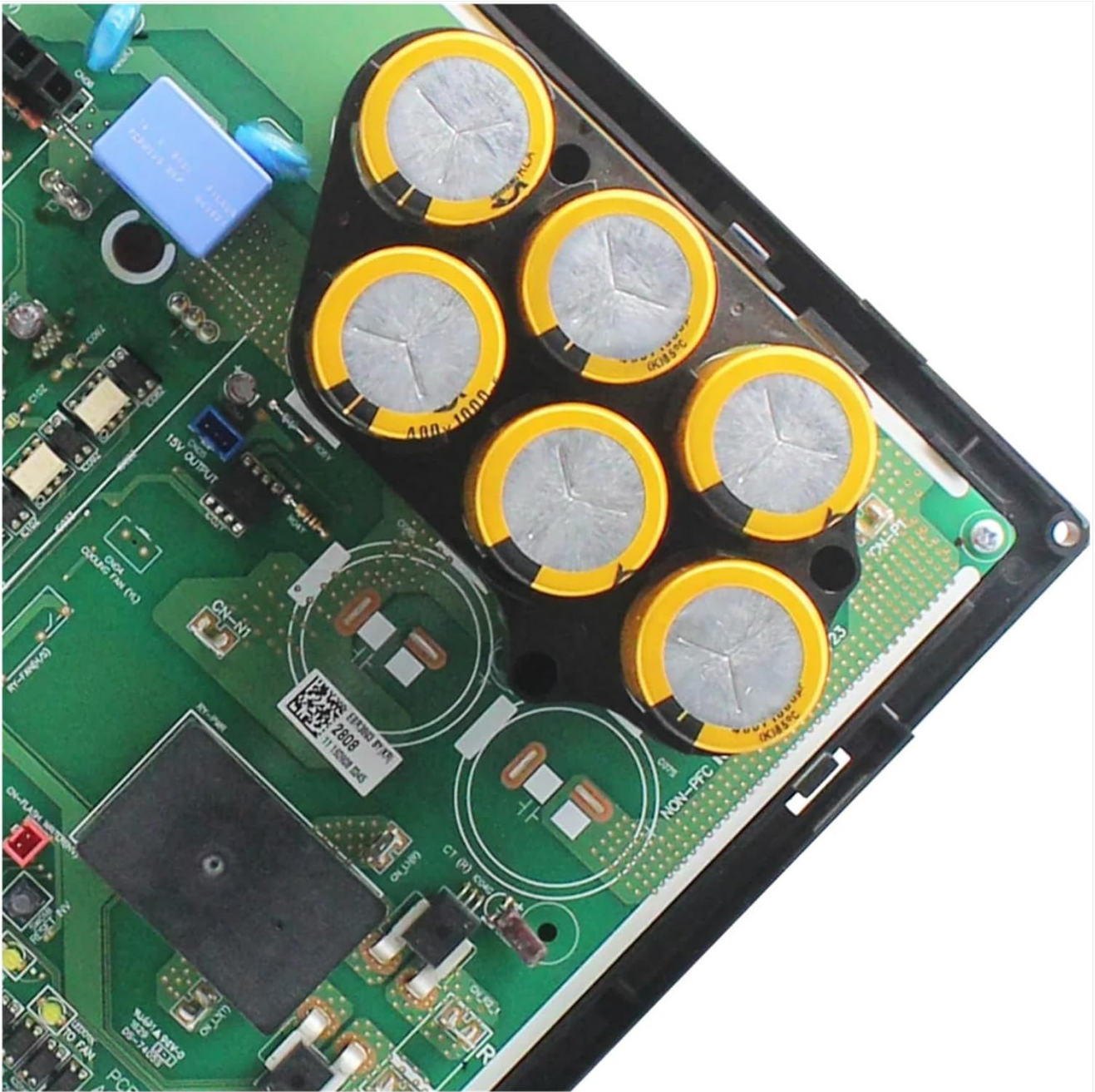
Figure 3: Close-up view of the power capacitors and central processing area on the PCB. These components are crucial for power regulation and the inverter's operation.
