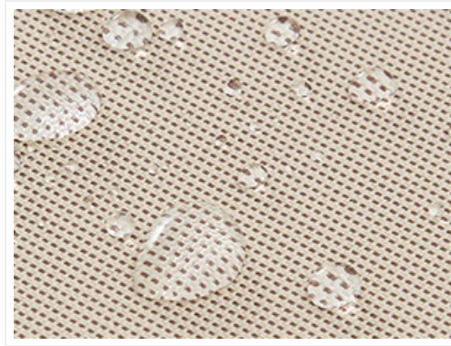
Image: A magnified view of the cushion fabric, demonstrating its waterproof properties with visible water droplets beading on the surface.
