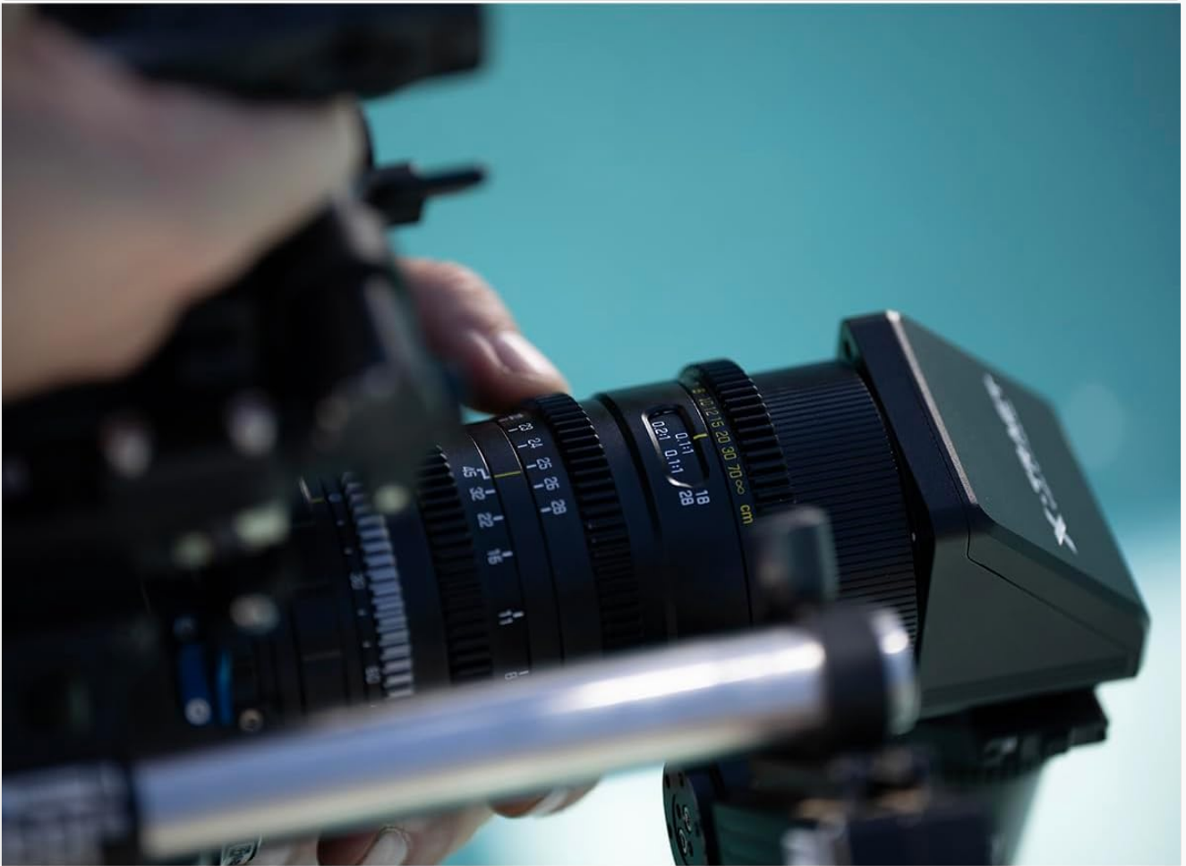
Figure 3: Detailed view of the manual control rings for focus, iris, and zoom.
