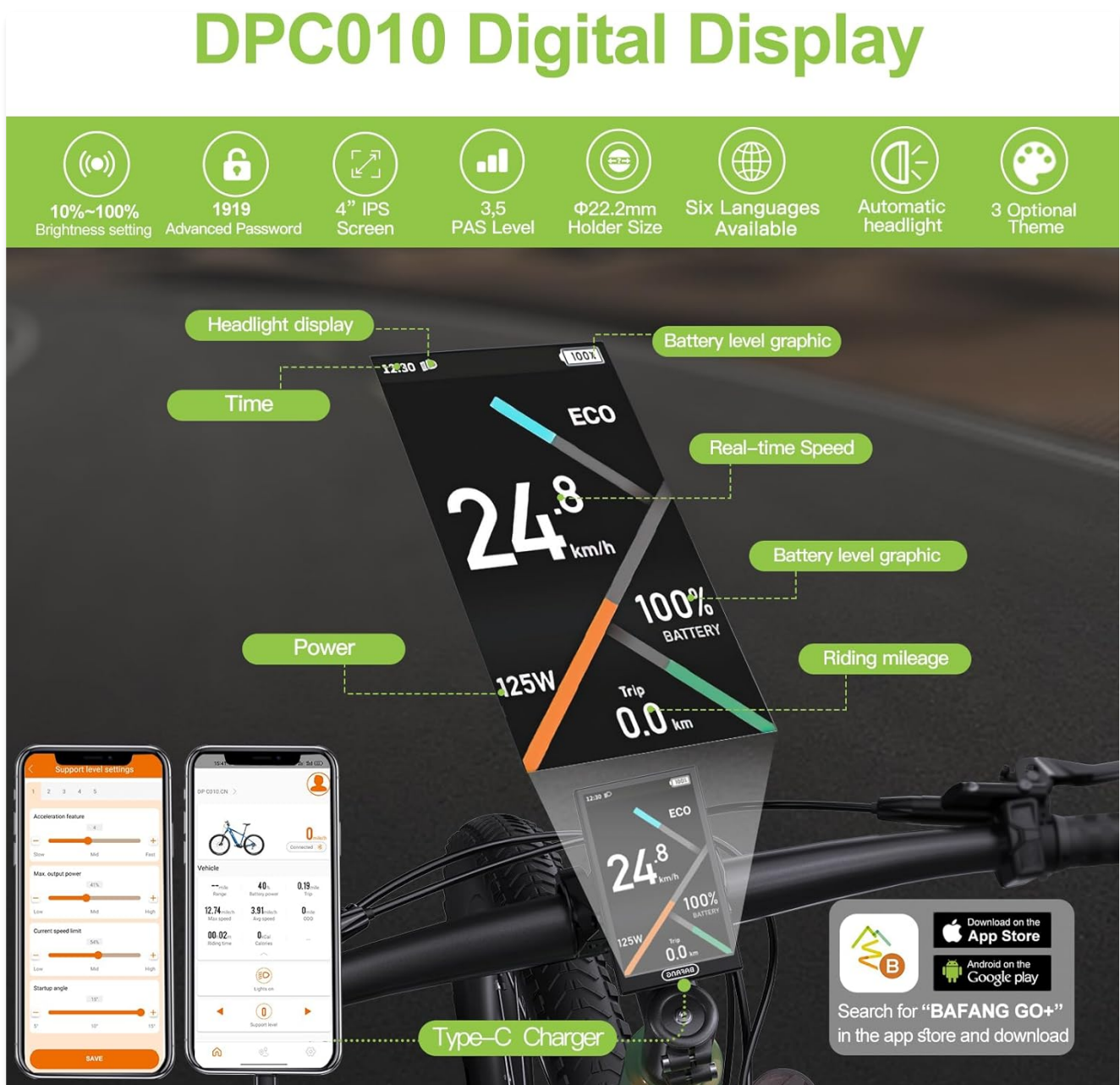
Figure 4.1: The DPC010 digital display interface showing various data points and app integration details.
