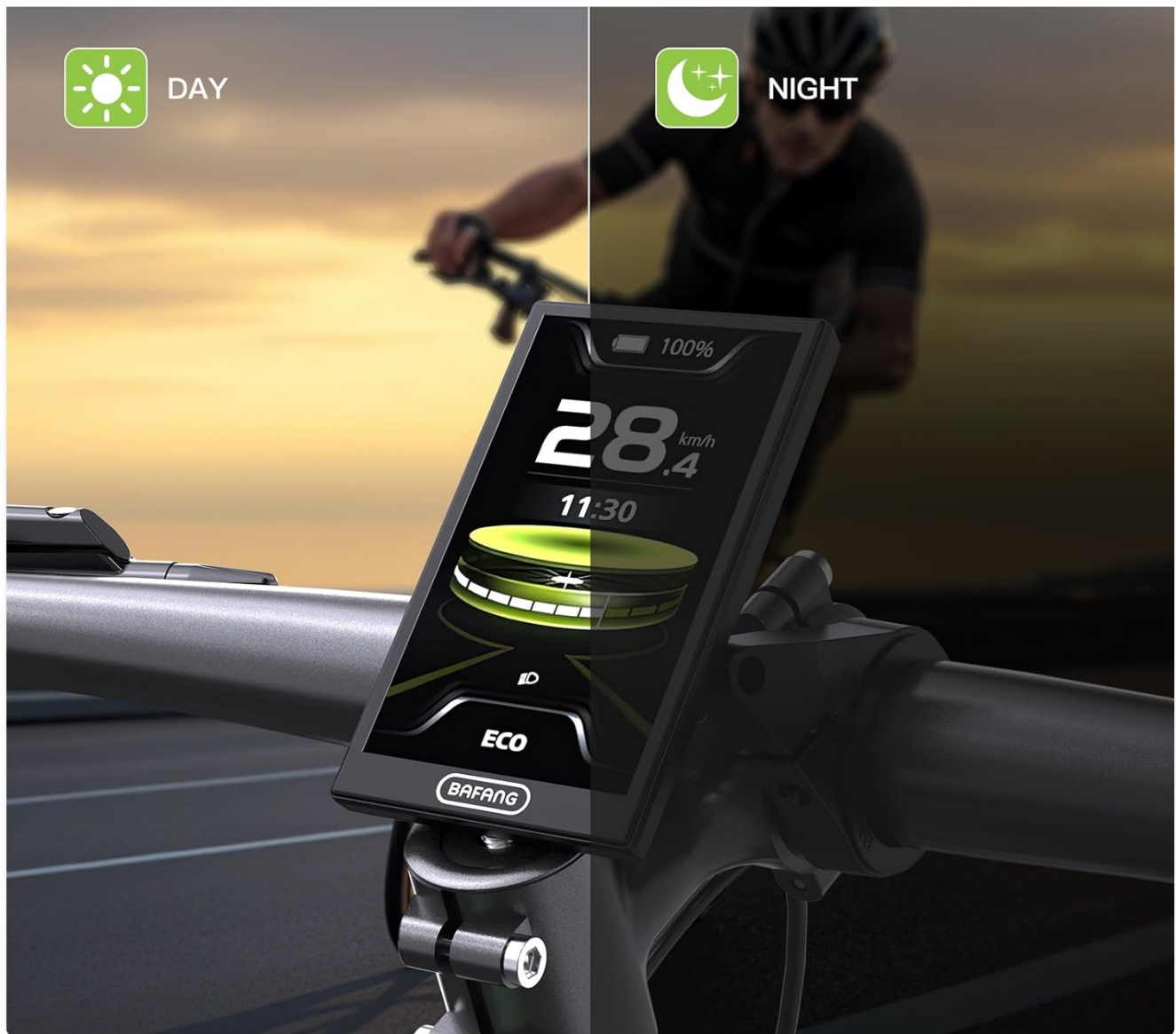
Figure 4.2: Comparison demonstrating the automatic backlight feature of the display in day and night conditions.
