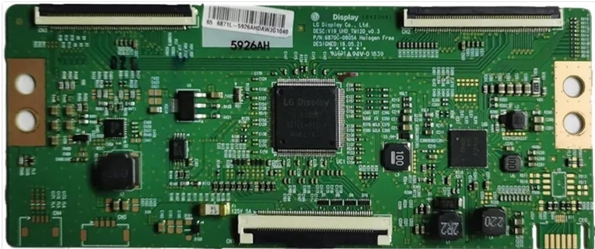
Image 1: Top view of the 6870C-0805A T-CON board, illustrating the layout of the main LG Display chip, capacitors, resistors, and connectors. This view helps in identifying the board and its primary components during installation.
