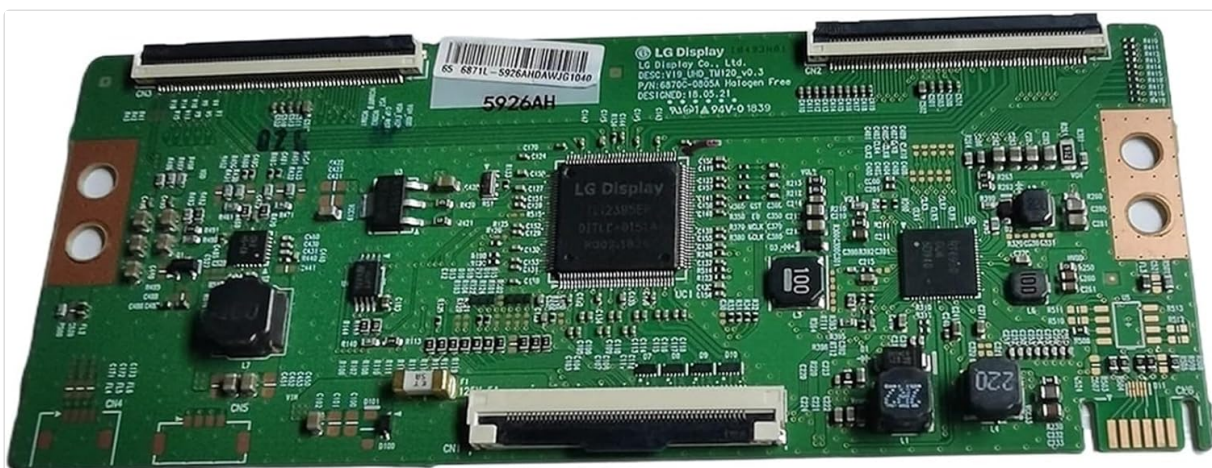
Image 2: An angled perspective of the 6870C-0805A T-CON board, providing a clearer view of the various connectors for ribbon cables and the general arrangement of surface-mounted components. This angle can assist in proper cable alignment.
