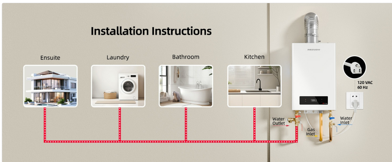
Figure 3: Overview of installation connections and potential indoor locations (Ensuite, Laundry, Bathroom, Kitchen).
