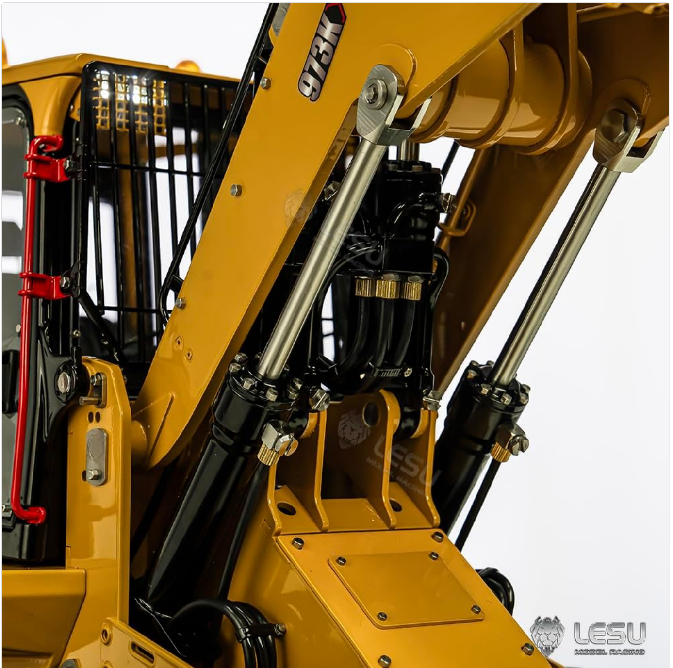
Figure 3: Detailed view of the hydraulic cylinders controlling the loader's movements.
