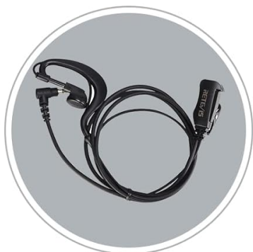
Figure 5: The Retevis B3H Walkie Talkie is compatible with 3.5mm 1-pin headphones, shown with an example earpiece and its connector.
