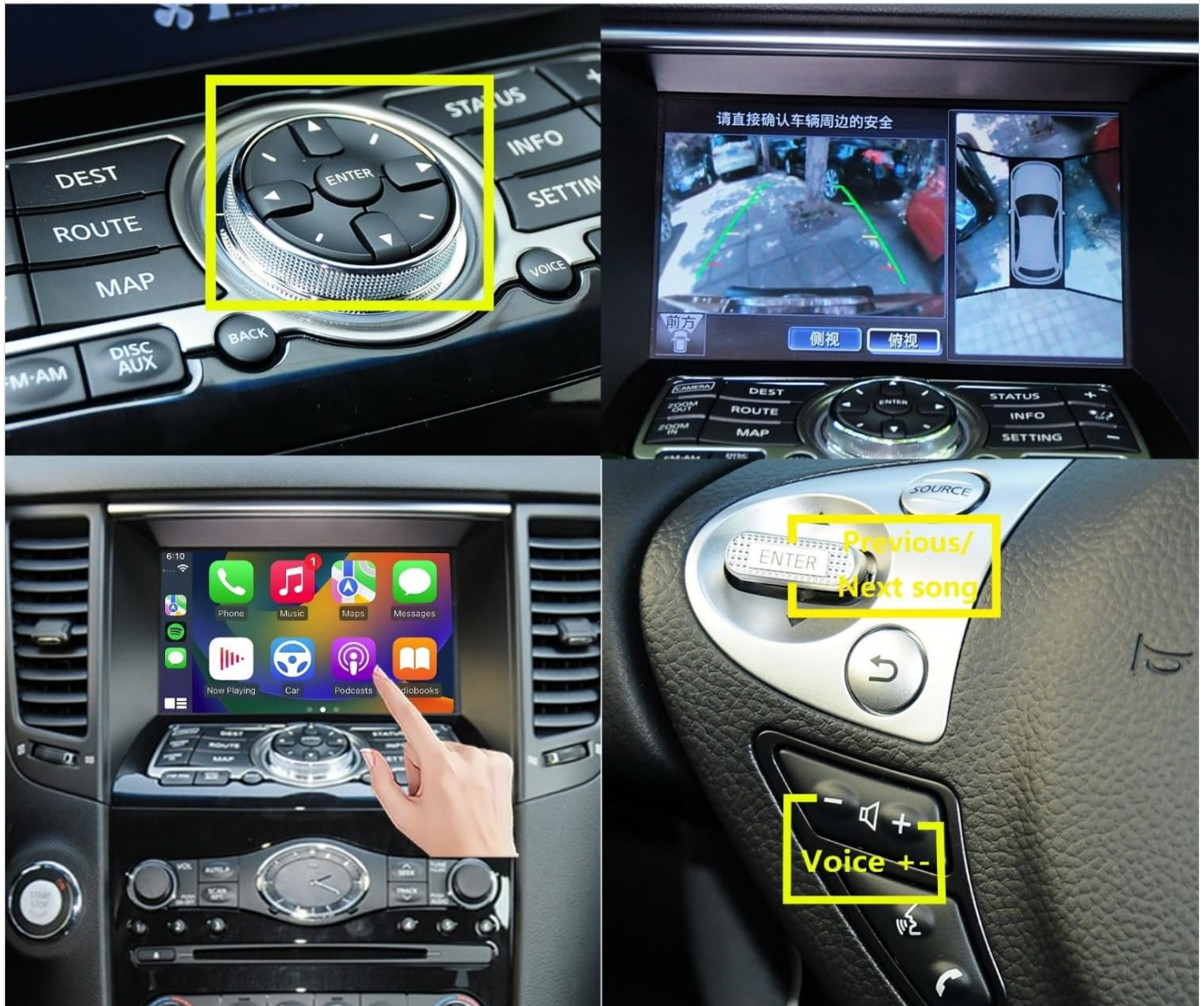
Image 5.2: Demonstrates the continued functionality of the vehicle's control knob, touchscreen, steering wheel controls, and original 360-degree camera system with the integrated module.
