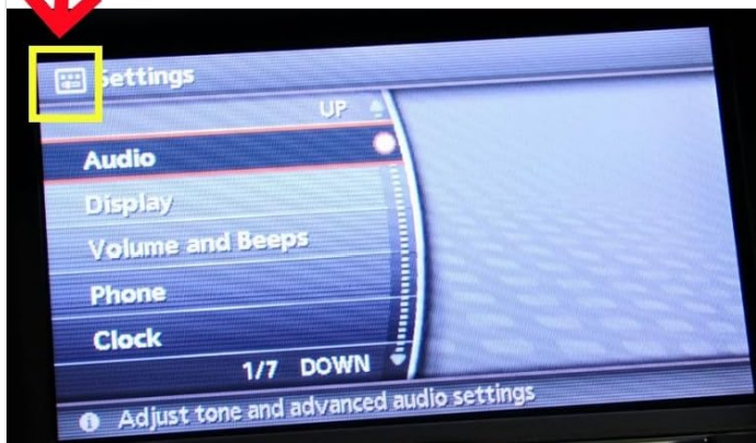
Image 2.1: Visual guide for checking screen compatibility. The right image shows a compatible screen (no icon next to 'Settings'), while the left image shows an incompatible screen (icon present).
