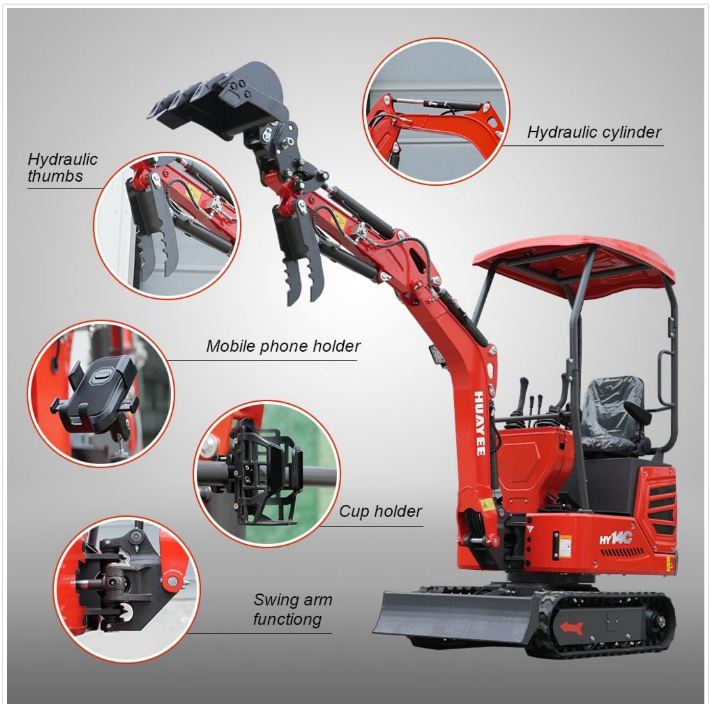
Figure 1: Key components of the HY14C Mini Excavator, highlighting the hydraulic thumbs, mobile phone holder, cup holder, swing arm function, and hydraulic cylinder.
