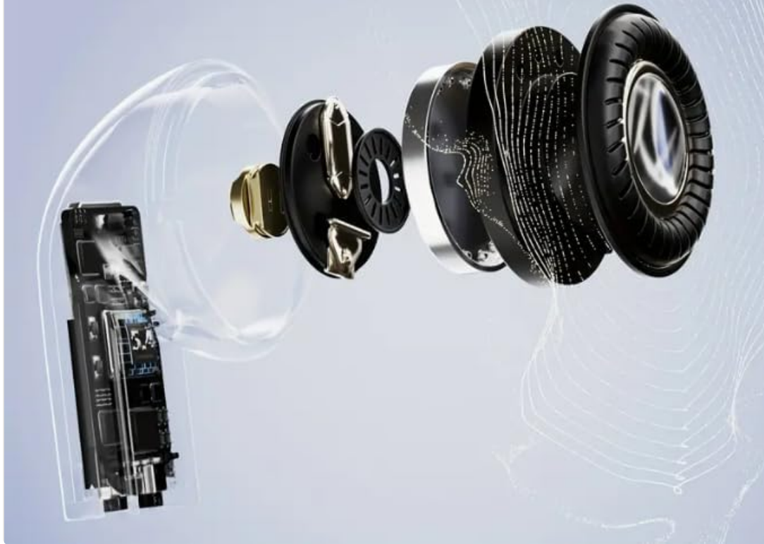
Figure 8: Internal components of the earbud, illustrating the high rebound ring diaphragm for enhanced sound.
