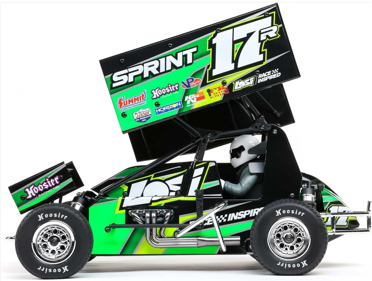
Image 1.2: Side profile of the 22S Sprint, highlighting the chassis, suspension, and large rear wing.
