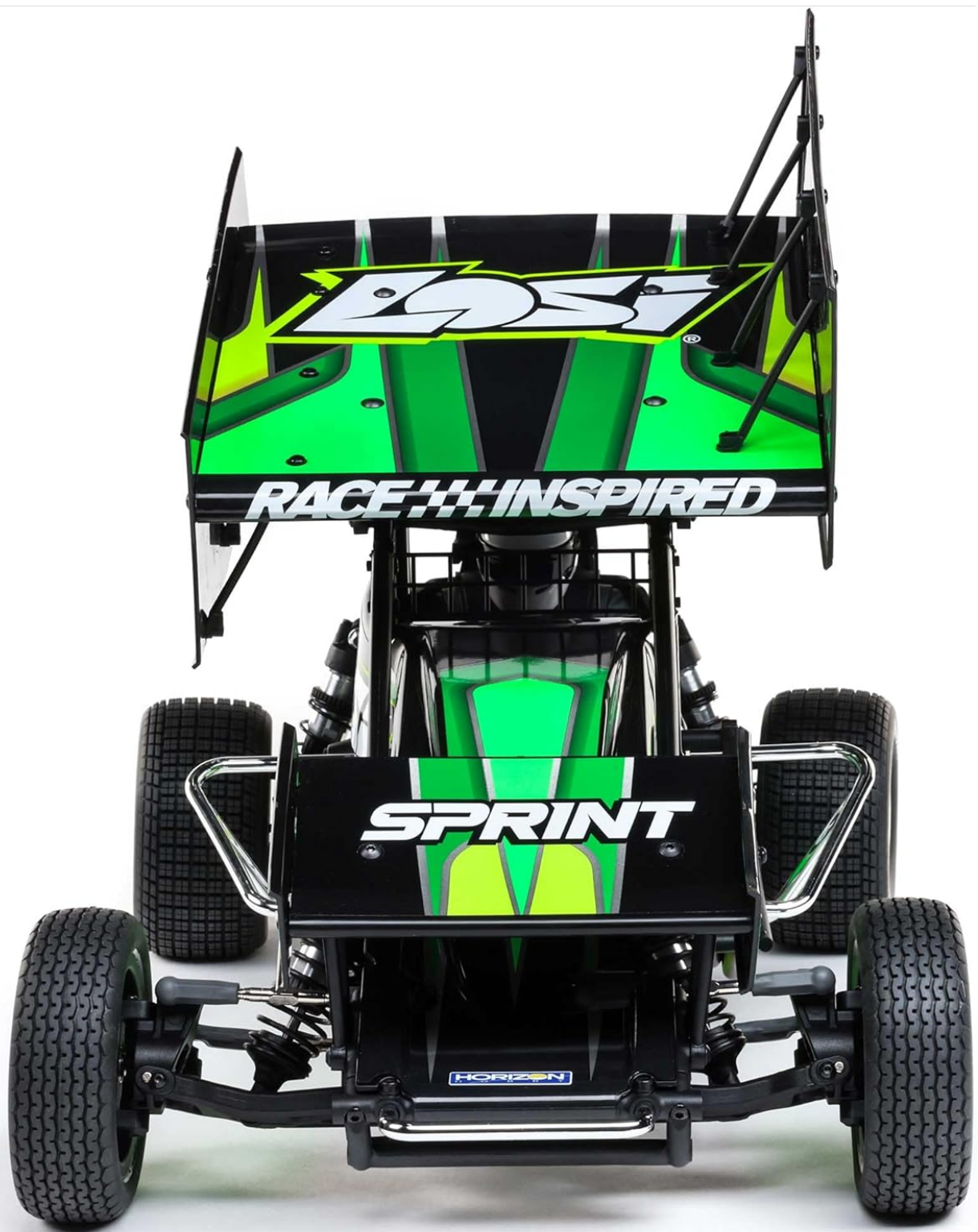
Image 1.3: Front view of the 22S Sprint, showing the front wing, suspension arms, and tire tread.
