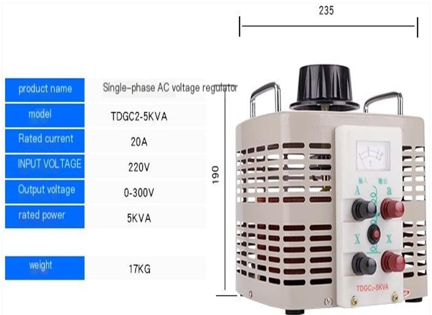
Figure 3.3: Side view of the PLPFUDVDZZ TDGC2-5KVA AC Power Regulator, illustrating its physical dimensions and a label detailing key specifications such as model, rated current, input/output voltage, and rated power.
