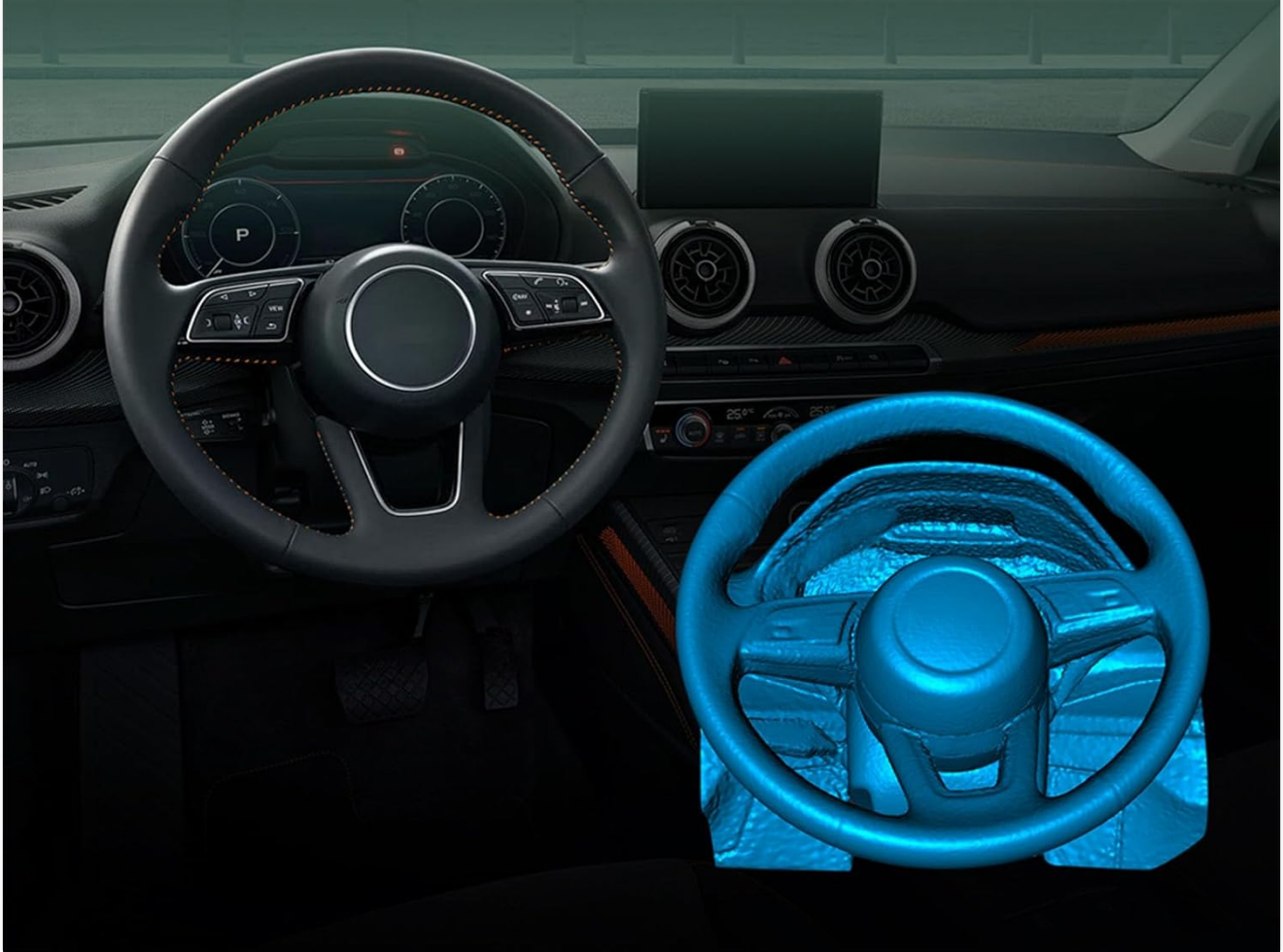
Figure 4.3: Scanning black or metallic objects without requiring spray.
