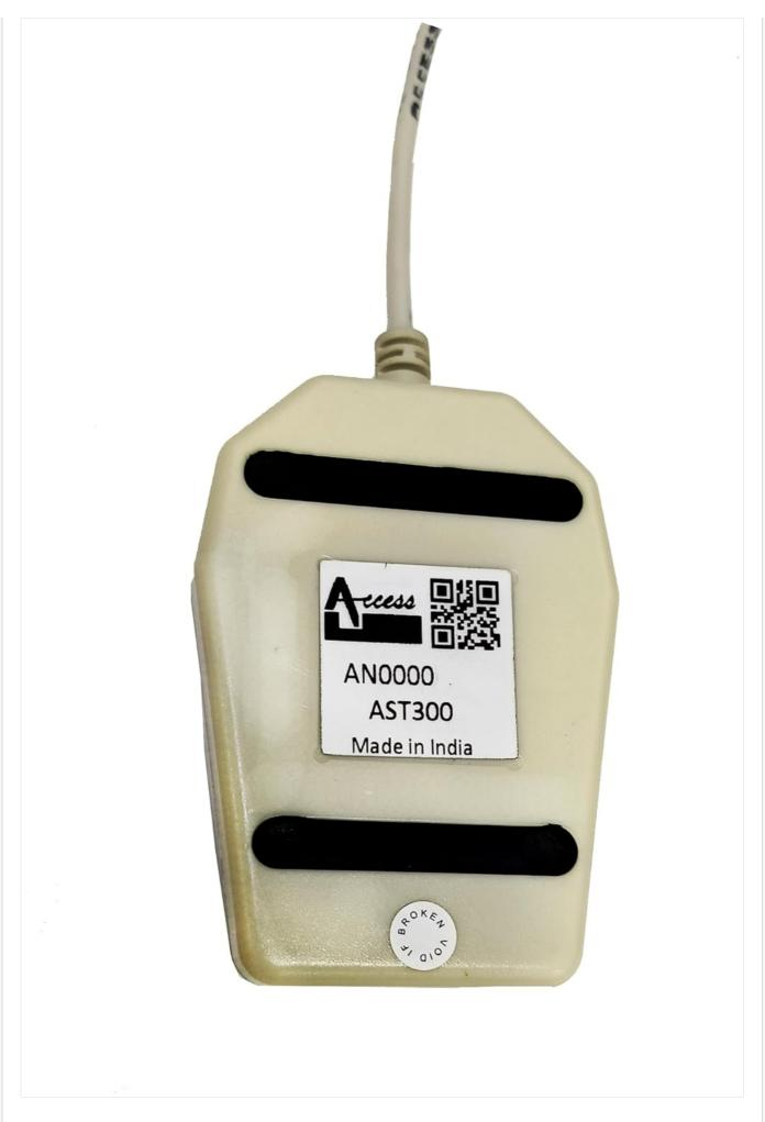
**Figure 2.2:** Rear view of the Access AST300 L1 Fingerprint Scanner, displaying the model number (AST300) and manufacturing details.
