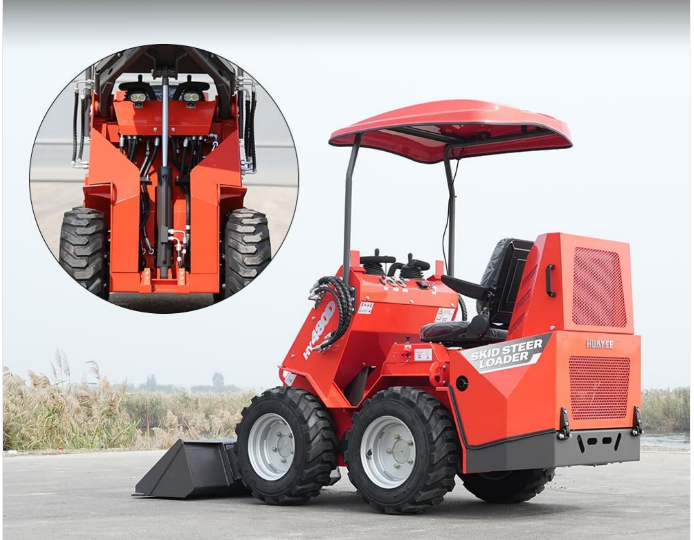
Image 4.2: The hydraulic cylinder system facilitates easy lifting and lowering of the arm.
