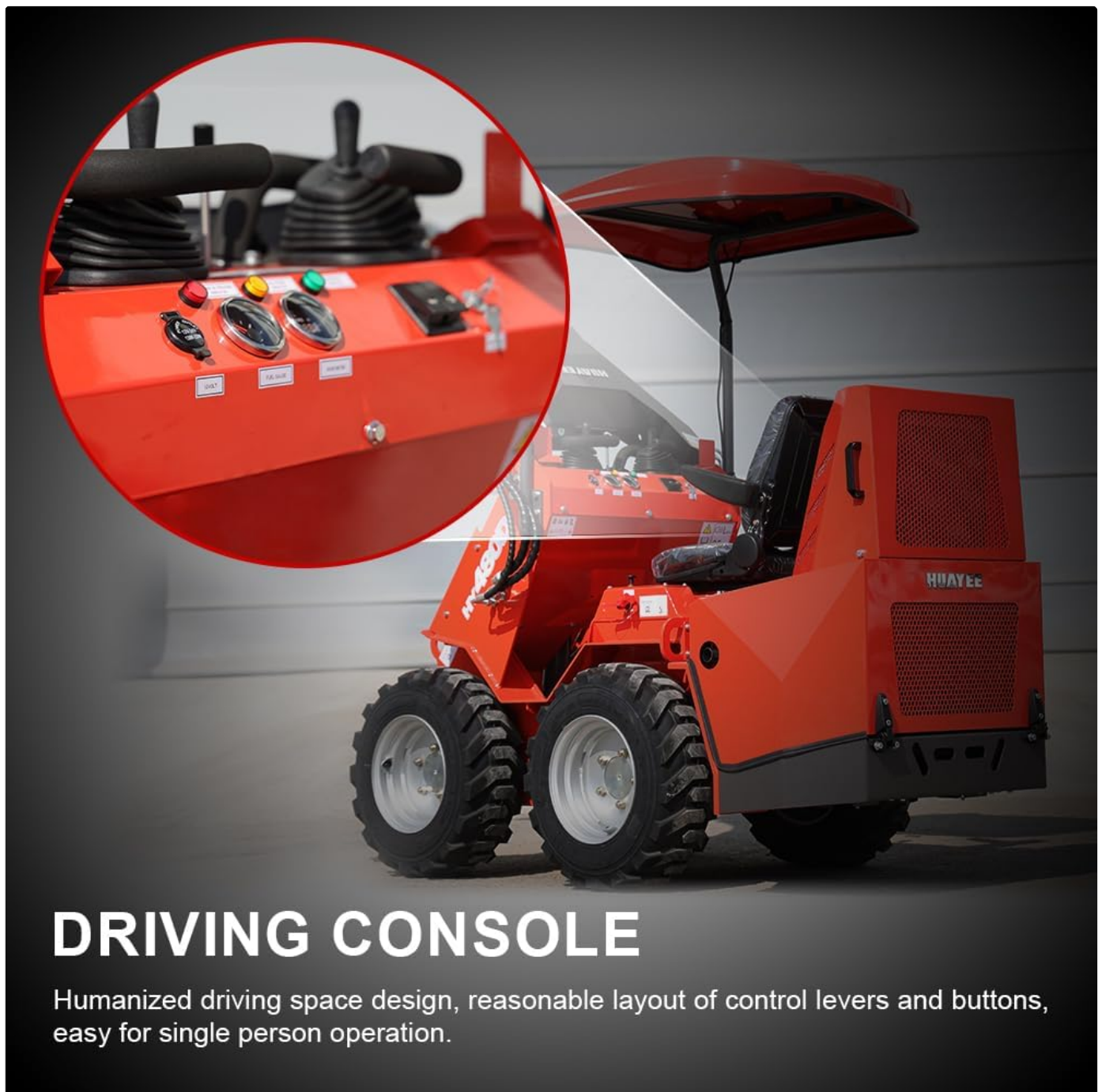
Image 3.2: Detailed view of the driving console, showing gauges and control switches.
