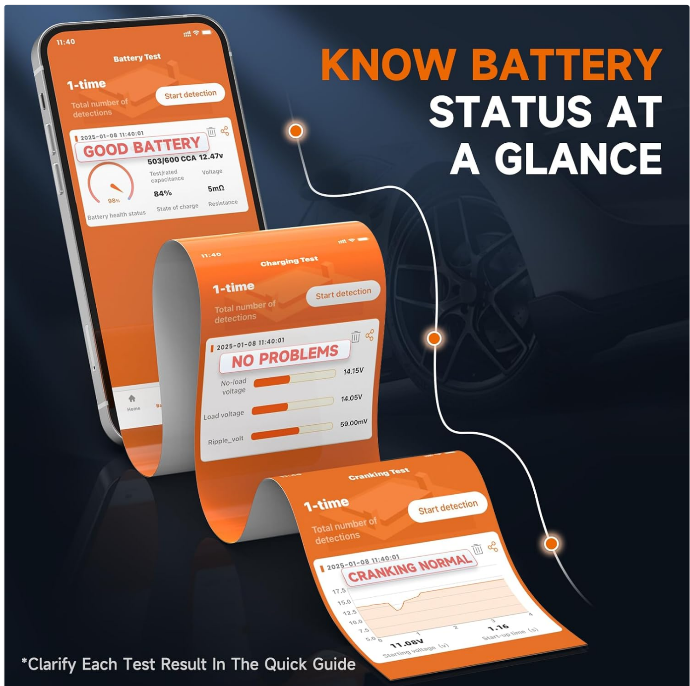
Image: Screenshots of the BT60 mobile app interface, showing how battery status, charging test results, and cranking test data are displayed for quick assessment.
