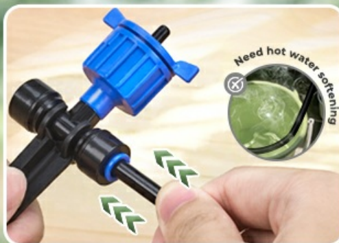
Image: Illustration of fully inserting the tube into the main unit's port by 15mm (5/8") to prevent pump failure.
