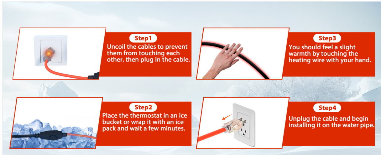
Image 5.1: Initial steps for preparing the heating cable.
