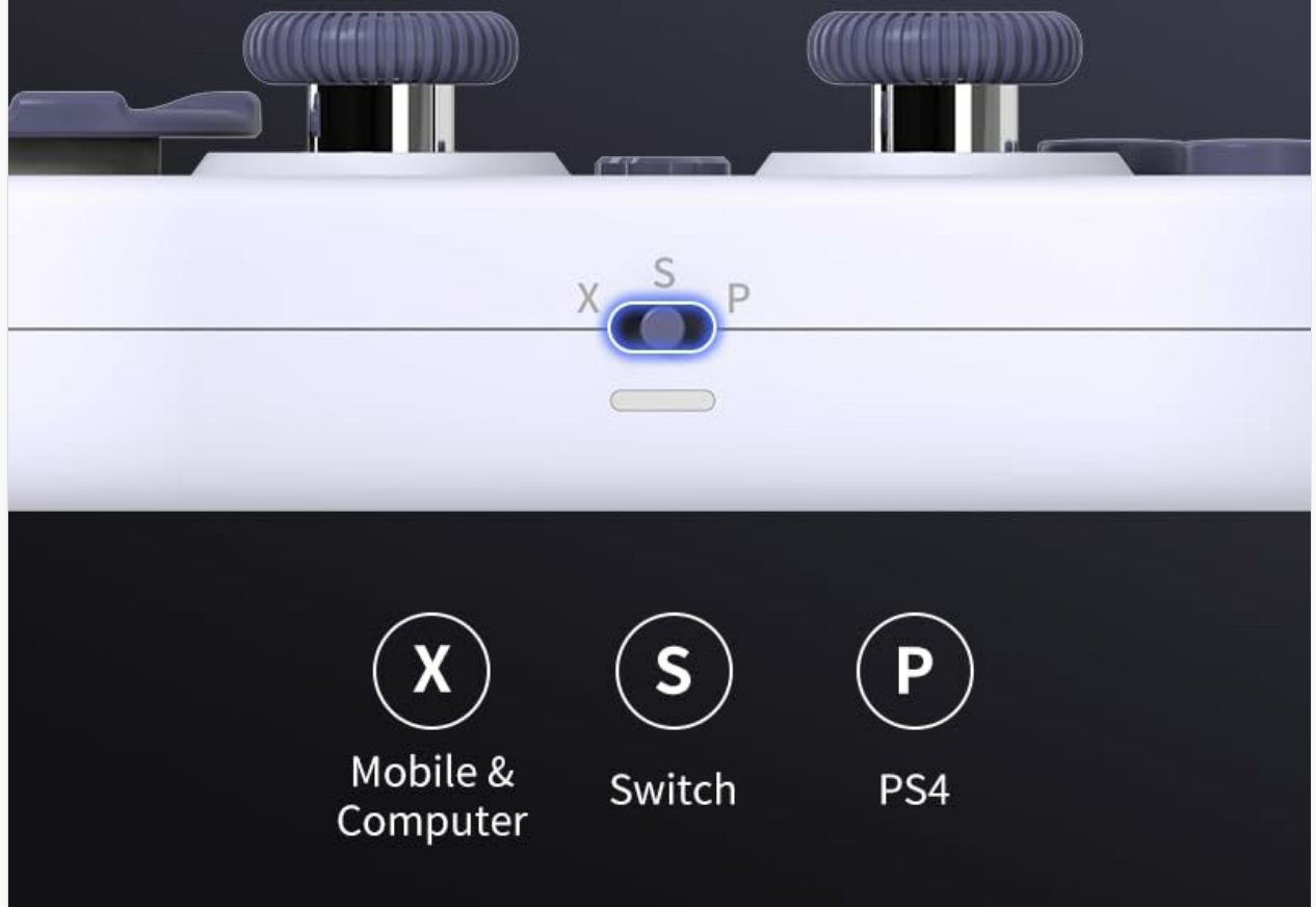
Image 3.2: Detail of the three-mode fast switching selector on the controller.
