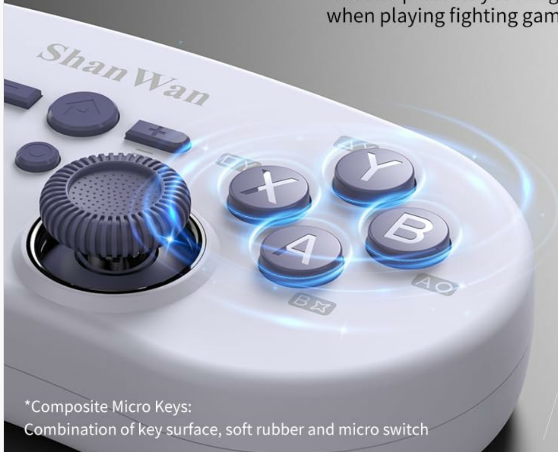
Image 4.2: Close-up of the composite micro-switch action buttons.
