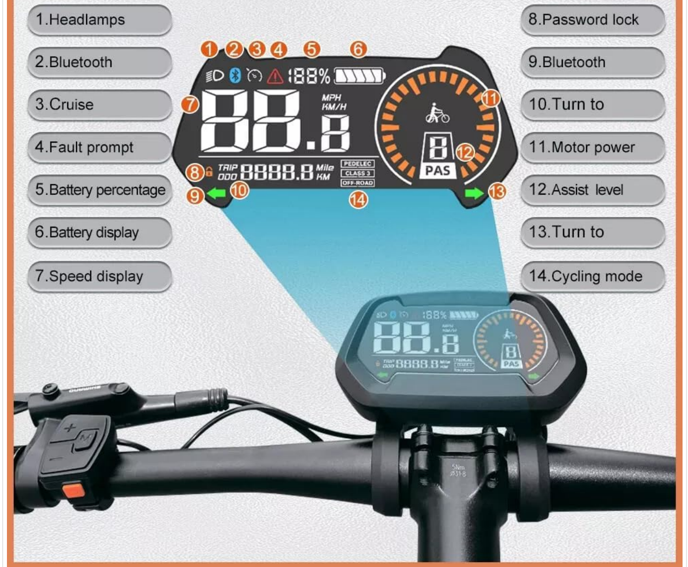
Figure 4: Detailed view of the DZ43 display's instrument features, indicating various data points and control indicators.
