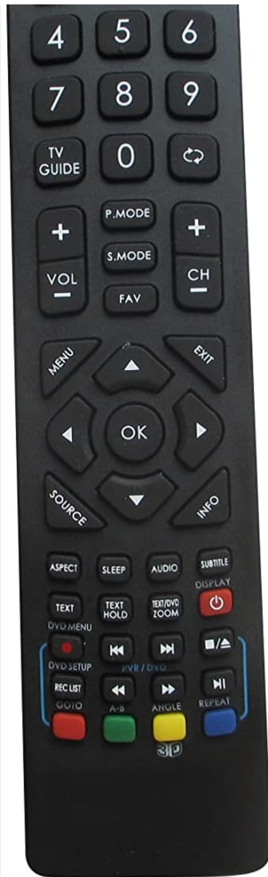
Figure 2.1: Front view of the remote control. This image displays the full button layout, including power, number keys, channel and volume controls, navigation pad, and various function buttons for TV, DVD, and media playback.
