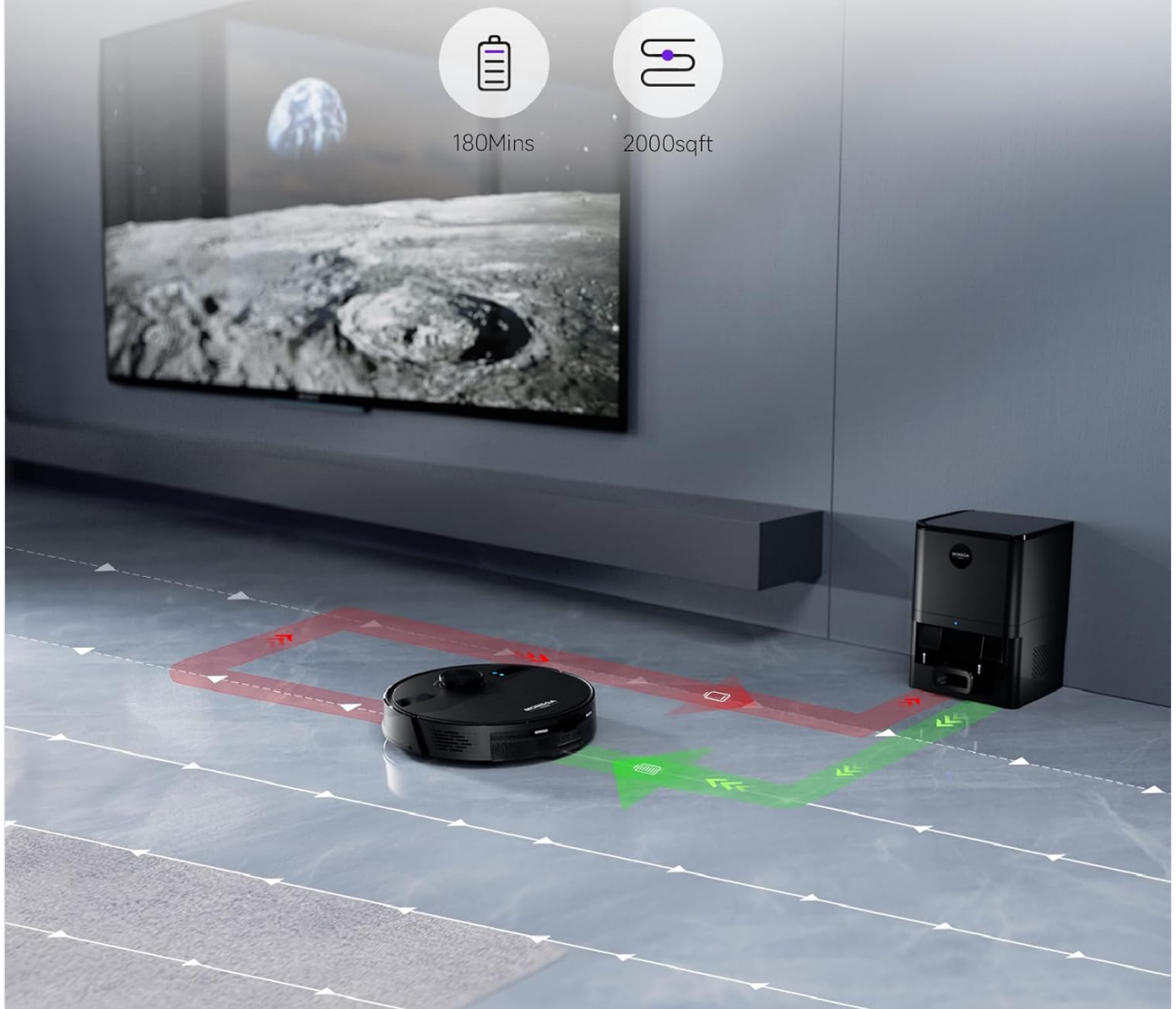
Figure 5.4: Auto recharge and resume cleaning function.
