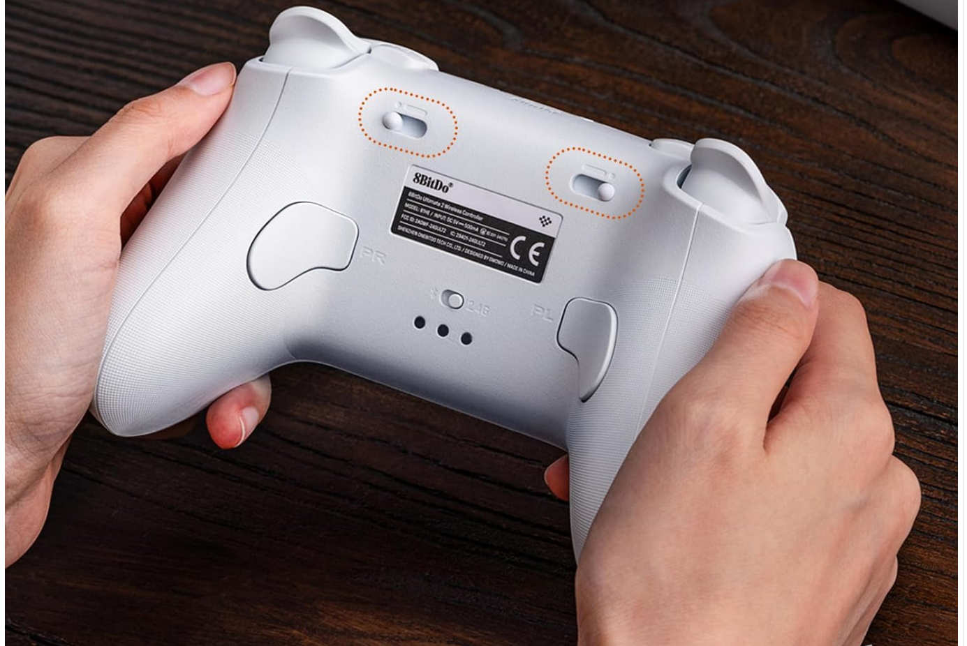
Figure 6: View of the controller's underside, highlighting the switches for dual trigger modes.
