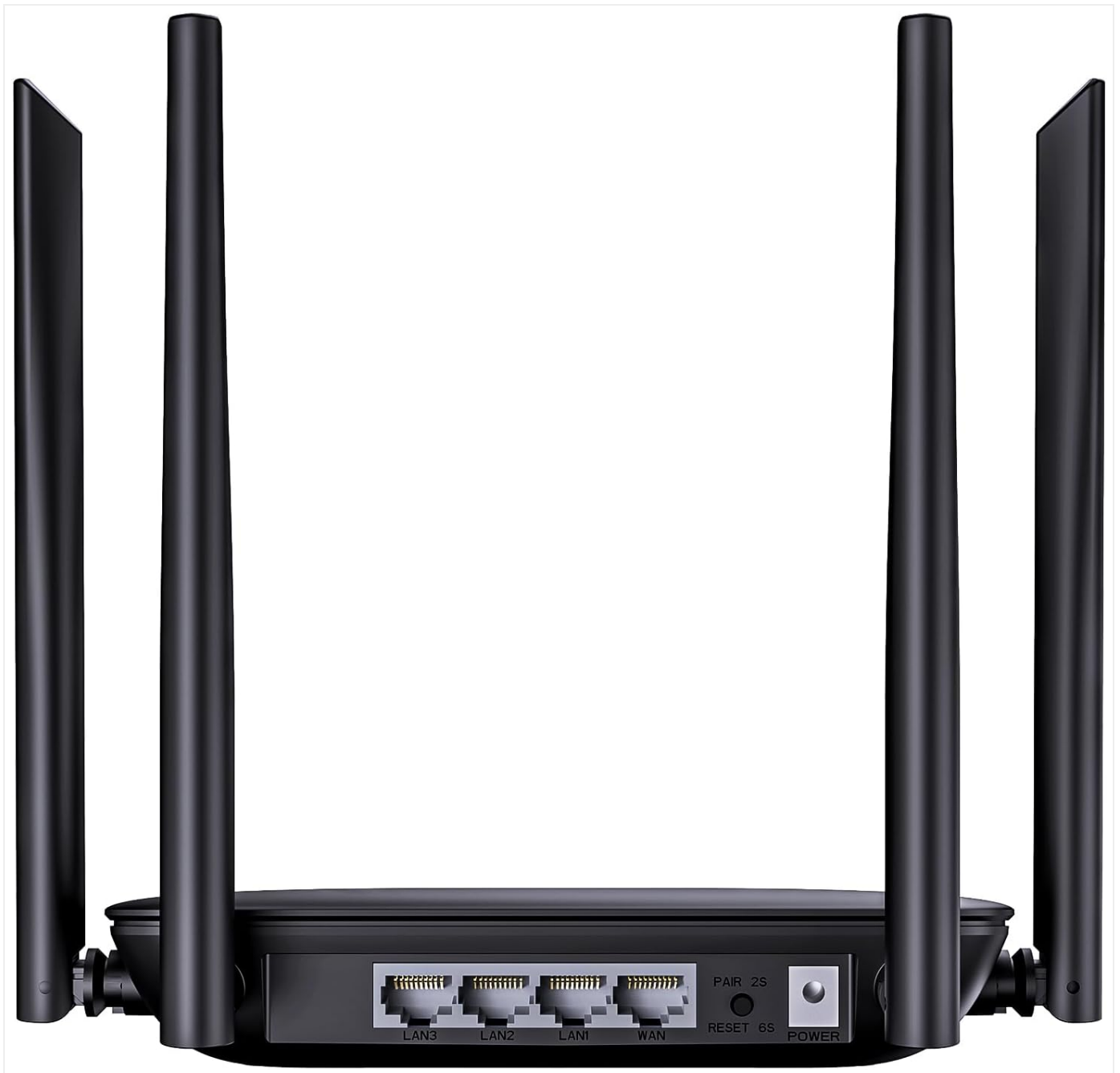
Figure 2: Rear view of the WAVLINK BE3600 WiFi 7 Router, showing WAN, LAN, Reset, and Power ports.
