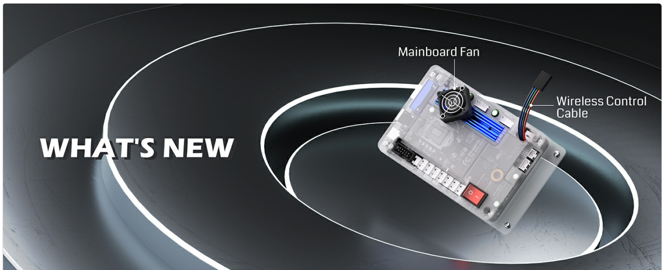
Figure 7: Image showing the upgraded motherboard with an integrated cooling fan for enhanced safety and stability.
